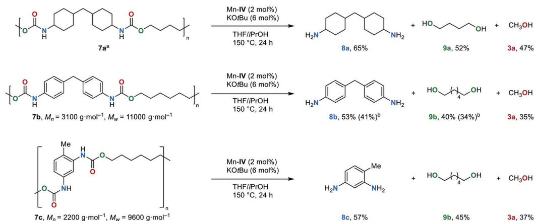
Fig. 5 First example on the transfer hydrogenation of polyurethanes **7** (0.5 mmol of substrate was used according to the repeating unit of polyurethanes). <sup>a</sup>Molecular weight could not be determined. <sup>b</sup>Isolated yield.
