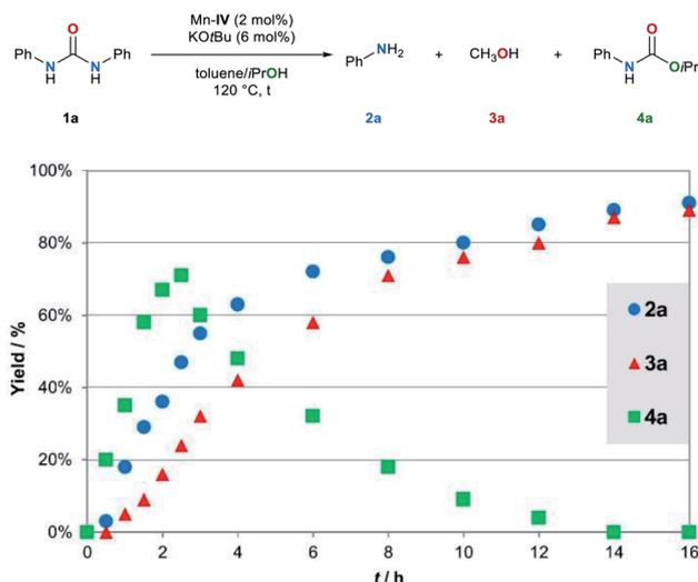
Fig. 2 Kinetic profile for the transfer hydrogenation of **1a**. Reaction conditions: **1a** (0.5 mmol), Mn-IV (2 mol%), KOtBu (6 mol%), toluene (1 mL), iPrOH (1 mL), 120 °C, 16 h. The yield was determined by GC using mesitylene as the internal standard.
