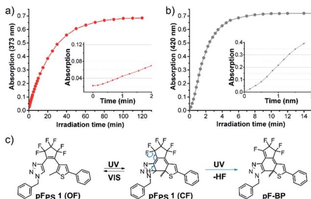
Fig. 8 Kinetic trace of absorption bands formed in **pF<sub>PS</sub> 1** solutions during UV light irradiation (310 nm, 60  $\mu$ M in (a) methanol (absorption band at 373 nm) and (b) DMSO (absorption band at 420 nm), (c) hypothetic reactions of **pF<sub>PS</sub> 1** in these solvents and the assumed structure of the specific side product **pF-BP**.
