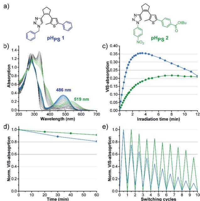
Fig. 12 Effect of structure optimization on the photochromic properties: (a) structures of **pHPS 1** and **pHPS 2**, (b) absorption spectra change of 60  $\mu\text{M}$  solutions of **pHPS 1** and **pHPS 2** during UV light irradiation (310 nm, LED) in DMSO to the (p)PSS, (c) kinetic trace of the VIS absorption bands during prolonged UV illumination, (d) thermostability (20  $^{\circ}\text{C}$ ), (e) reversibility measurement (normalized VIS absorption).
