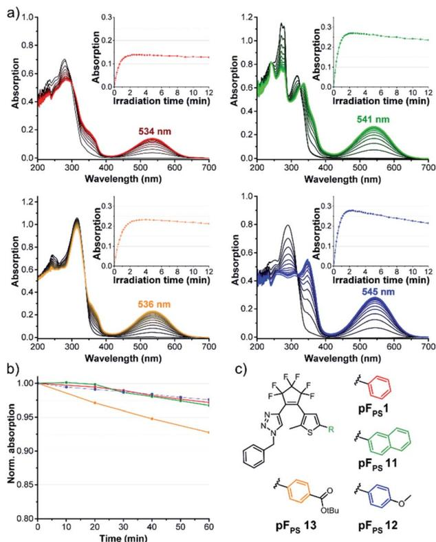
Fig. 5 Photochromic properties of various thieryl substitutions: (a) time-dependent changes of the absorption spectra of 60  $\mu\text{M}$  solutions of pF<sub>PS</sub> 1, 11–13 upon UV light irradiation (310 nm, LED) in chloroform towards the (pseudo)-photostationary state; insets show the absorption vs. time trace measured at the VIS absorption maximum during extended UV irradiation to analyse the photostability, (b) thermostability (20 °C) of the CF isomers, (c) structures.
