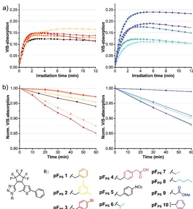
Fig. 4 Comparison of the photochromic properties of various alkyl triazole photoswitches **pFps 1–10** (60  $\mu\text{M}$  solutions in chloroform): (a) kinetic trace of the absorbance at the VIS maximum, (b) thermostability (20  $^\circ\text{C}$ ) of the closed-ring forms.
