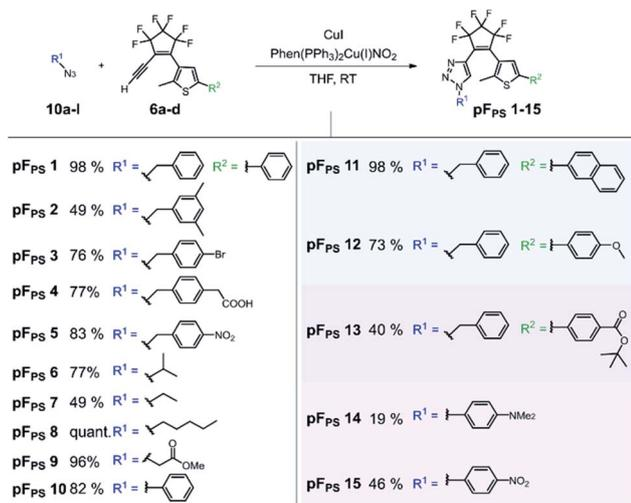
Scheme 2 CuAAC reaction yields of perfluorocyclopentene acetylene precursors (**6a–d**) with small organic azides (**10a–l**). 15 different triazole photoswitches were synthesized (**pF<sub>PS</sub> 1–15**).
