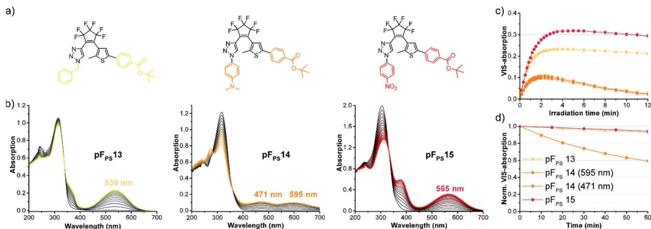
Fig. 6 Effect of electron-donating and electron-withdrawing substituents at the triazole ring on the photochromic properties: (a) structures of pF<sub>PS</sub> 13–15, (b) time-dependent changes of the absorption spectra of solutions (60  $\mu\text{M}$  in  $\text{CHCl}_3$ ) during UV light irradiation (310 nm UV light) to the (pseudo)-photostationary state, (c) kinetic trace of the VIS absorption bands during extended UV irradiation, (d) thermostability (20 °C) of the CF isomers.
