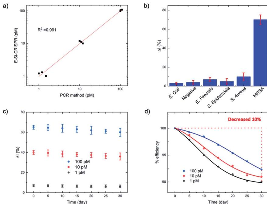
Fig. 5 (a) Comparison of *mecA* concentrations between the E-Si-CRISPR and PCR at 1, 10 and 100 pM. (b) Specificity test for MRSA versus other bacteria for the E-Si-CRISPR technique, revealing excellent specificity ( $N = 3$ ). (c and d) Stability of the ssDNA-immobilized electrode for detecting *mecA* (1, 10 and 100 pM) over 30 days ( $N = 3$ ).
