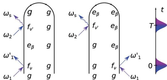
Fig. 3 Loop diagrams for the SXRS signal.
