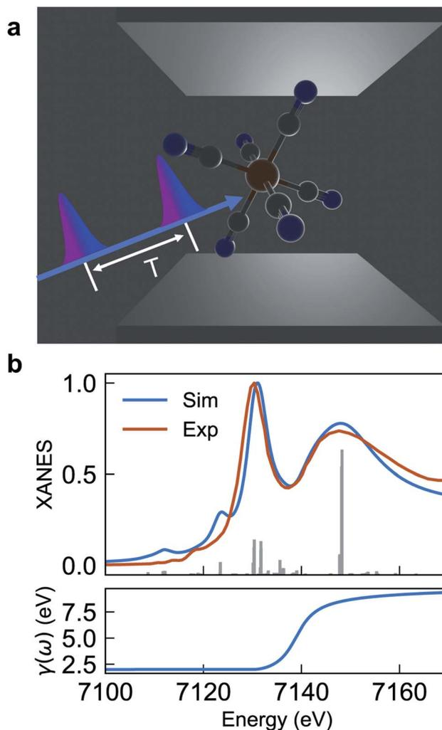
Fig. 1 (a) Schematic of  $[\text{Fe}(\text{III})(\text{CN})_6]^{3-}$  molecules embedded in an optical cavity and pulse sequence used in the SXRS signal. The cavity length is in the  $\mu\text{m}$  scale for UV/Vis cavities, and nm scale for X-ray cavities. (b) Comparison of experimental and simulated XANES spectrum eqn (2) (upper panel) and frequency-dependent broadening function (lower panel). The simulated spectrum is blueshifted by 142 eV to fit experiment.
