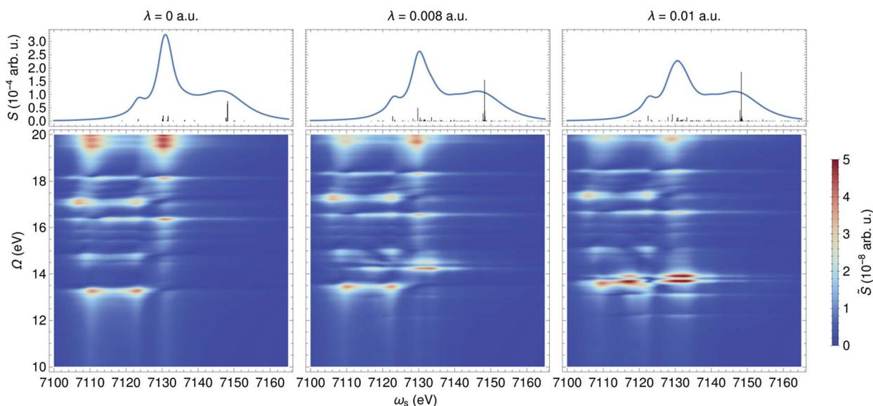
Fig. 4 XANES (top) and SXRS (bottom) of ferricyanide embedded in an optical cavity with frequency  $\omega_c = 8$  eV and varying coupling strengths  $\lambda$ . The bipolariton states are clearly observed in the SXRS spectra.
