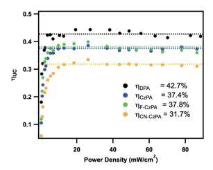
Fig. 5 Upconversion quantum efficiencies measured for 0.25 mM acceptors/annihilators sensitized by  $Zr(^{Mes}PDP^{Ph})_2$  ( $OD_{514\ nm}=0.2$ ) in deaerated THF solutions as a function of excitation power density at 514.5 nm.
