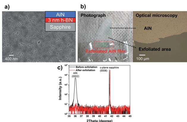
Fig. 4 (a) A top-view SEM image of the grown AlN at 1380 °C on h-BN/*c*-plane Al<sub>2</sub>O<sub>3</sub>. (b) Photographic and optical microscopy images showing the exfoliated AlN film caused by the interfacial h-BN layer. (c) XRD 2 $\theta$ - $\omega$  scans of the AlN layer before and after exfoliation.
