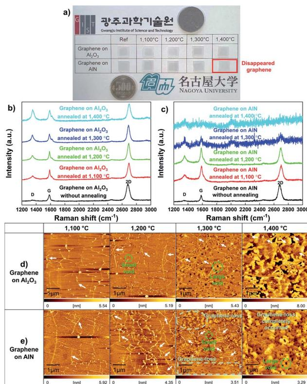
Fig. 1 (a) Photographs of annealed graphene on  $Al_2O_3$  and AlN at each temperature. The black sheet is graphene and can be distinguished by the naked eye. At 1400 °C, graphene-loss only occurred completely on AlN. Raman spectra of (b) graphene on  $Al_2O_3$  and (c) graphene on AlN annealed at each temperature. AFM images of annealed graphene at each temperature (d) on  $Al_2O_3$  and (e) on AlN. The white arrows indicate graphene wrinkles.
