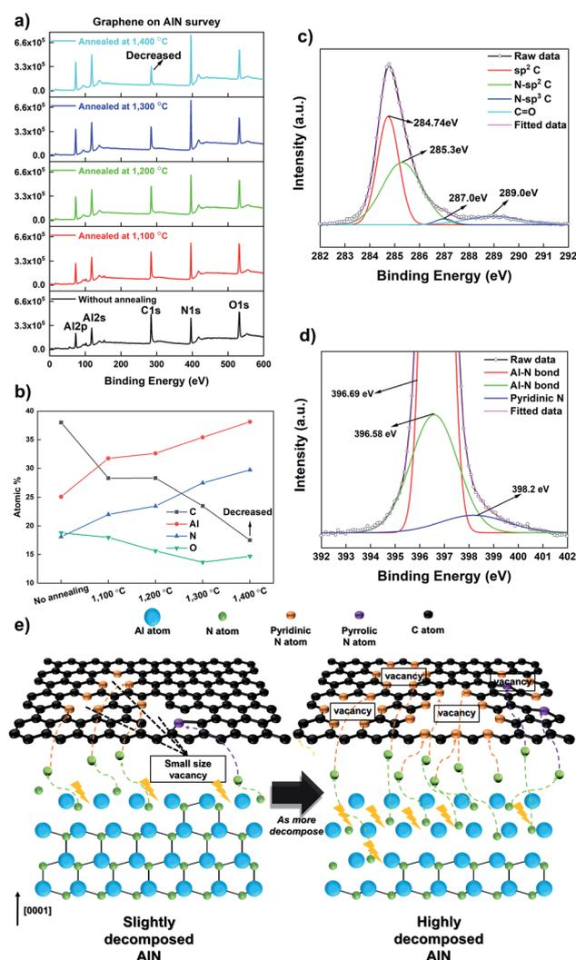
**Fig. 2** The influence of the N atom generated from substrate decomposition on graphene. (a) XPS spectra of annealed graphene on AlN showing the Al 2p, Al 2s, C 1s, N 1s, and O 1s peaks. (b) The total atomic percentage values of annealed graphene/AlN at the surface. (c) C 1s and (d) N 1s XPS spectra of the annealed graphene on AlN at 1300 °C revealing the signals of C–N bonding. (e) A schematic diagram of the graphene structure affected by the N atom depending on the AlN decomposition.
