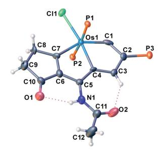
Fig. 3 X-ray crystal structure of the cation of 2c (thermal ellipsoids are set at the 50% probability level and the phenyl groups in the PPh<sub>3</sub> moieties are omitted for clarity). Selected bond lengths [A] and angles [°]: Os1-C1: 1.818(10), Os1-C4: 2.146(7), Os1-C7: 2.057(8), C1-C2: 1.411(12), C2-C3: 1.415(11), C3-C4: 1.394(10), C4-C5: 1.411(11), C5-C6: 1.427(11), C6-C7: 1.356(11), C5-N1: 1.387(11), N1H···O1: 2.107, H3···O2: 2.105 C4-Os1-C1: 72.6(3), C7-Os1-C4: 75.7(3)
