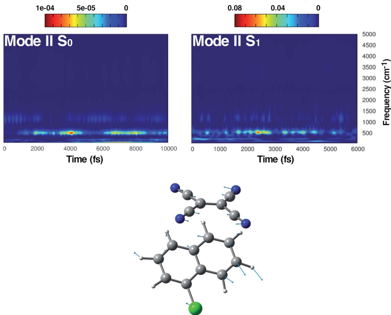
Fig. 5 Time resolved wavelet spectra of the symmetric in plane CCN bending (Mode II) extracted from the ground (left, 10 ps) and the excited state (right, 6 ps) trajectory. The magnitude  $|W(v,t)|^2$  of the wavelet power spectrum is reported as a color scale on the top.
