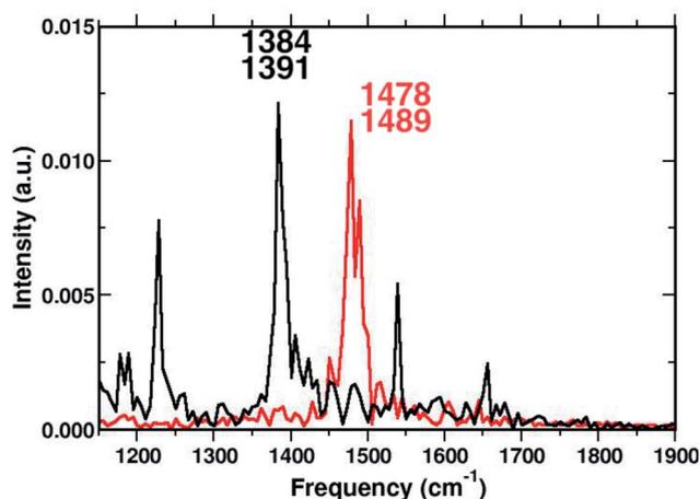
Fig. 7 Time-independent spectrum in the 1150–1900  $\text{cm}^{-1}$  spectral region, computed by the Fourier transform of the CC1 (black trace) and C=C (red trace) bond lengths averaged from the excited state AIMD trajectories.
