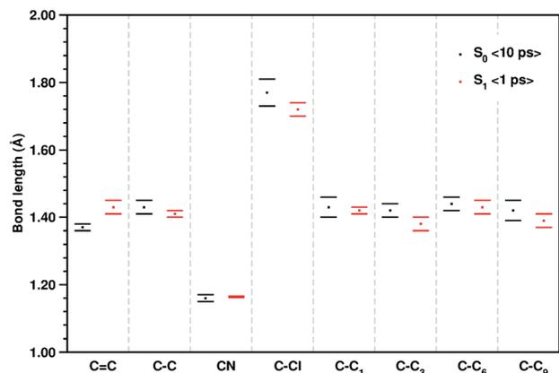
Fig. 3 Mean values of the selected structural parameters of the TCNE:1ClN CT complex, extracted from 10 ps  $S_0$  and the last 1 ps  $S_1$  AIMD trajectories. Labels are referred to Fig. 1, bond lengths are reported in Angstroms ( $\text{\AA}$ ), and standard deviations are given as error bars.
