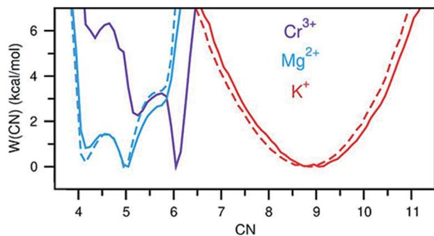
Fig. 4 Free energy as a function of coordination number of  $\text{Cr}^{3+}$ ,  $\text{Mg}^{2+}$ , and  $\text{K}^+$ . Solid and dashed lines indicate the KCl-MgCl<sub>2</sub> salt mixtures with and without  $\text{Cr}^{3+}$ , respectively.
