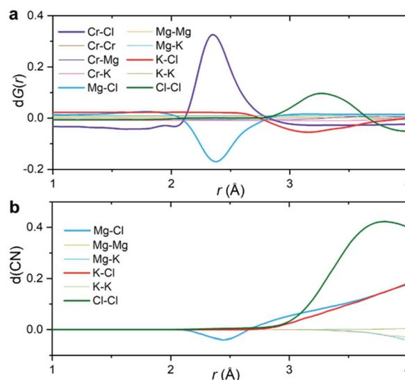
Fig. 3 Interpretation of the differential PDF. (a) Partial subcomponents of  $dG(r)$  from AIMD simulations. (b) Differential coordination number  $d(\text{CN})$  for the solvent–solvent correlations, showing the difference between the cumulative coordination number in the CrCl<sub>3</sub> loaded system and the pristine KCl–MgCl<sub>2</sub> molten salt.
