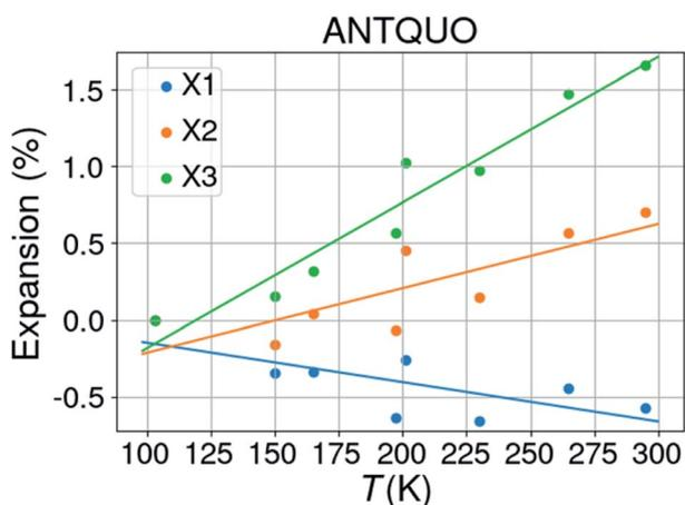
Fig. 5 Thermal expansion of anthraquinone.
