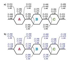
Fig. 6 Selected C–C bond lengths (a) and bond orders (b) calculated for rings A, B, and C (PBE0/cc-pVTZ) in  $\mathbf{1}^0$ ,  $\mathbf{1}^{2-}$  (round brackets), and  $\mathbf{1}^{4-}$  [square brackets].
