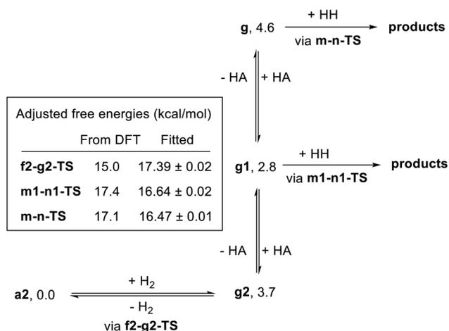
Fig. 11 Optimized kinetic model. The free energies of **a2**, **g2**, **g1**, and **g** were held fixed at the indicated values. The free energies of **f2-g2-TS**, **m-n-TS**, and **m1-n1-TS** were adjusted to achieve the best global fit to the kinetic data. HH refers to hexyl hexanoate and HA refers to 1-hexanol.
