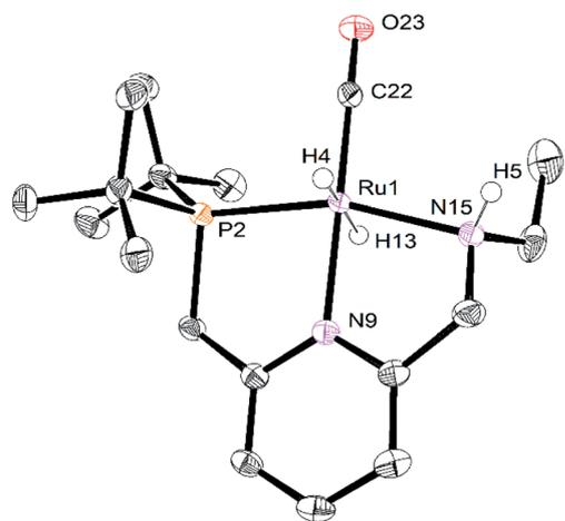
Fig. 6 ORTEP diagram of  $\text{RuPNN}^{\text{HEt}}$ , showing 50% probability ellipsoids. Hydrogen atoms other than Ru–H and N–H are omitted for clarity. Selected bond lengths (Angstroms) and angles (degrees): Ru(1)–P(2), 2.2536(6); Ru(1)–N(15), 2.1893(19); Ru(1)–N(9), 2.0980(19); Ru(1)–C(22), 1.830(2); C(22)–O(23), 1.164(3); P(2)–Ru(1)–N(9), 82.45(6); N(9)–Ru(1)–N(15), 78.71(7).
