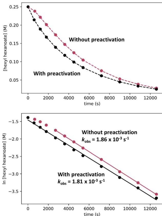
Fig. 8 Comparison of hexyl hexanoate hydrogenation catalyzed by  $\text{RuPNN}^{\text{imine}}$  with and without preactivation of the catalyst by incubation under 20 bar hydrogen for 90 minutes. The top plots show  $[\text{ester}]$  vs. time; dashed lines are merely to guide the eye and do not represent a fit to the data. The bottom plots show  $\ln[\text{ester}]$  vs. time, with linear fits to all data (with preactivation) or to the time points from 45 minutes on (without preactivation).
