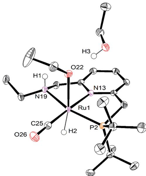
Fig. 7 ORTEP diagram of  $\text{RuPNN}^{\text{HOEt}}$ , showing 50% probability ellipsoids. Hydrogen atoms other than Ru–H, N–H, and O–H are omitted for clarity. Selected bond lengths (Angstroms) and angles (degrees): Ru(1)–P(2), 2.2671(5); Ru(1)–N(13), 2.1056(14); Ru(1)–N(19), 2.1693(14); Ru(1)–O(22), 2.1980(12); Ru(1)–C(25), 1.8357(19); C(25)–O(26), 1.159(2); H(1)–O(22), 1.725; H(3)–O(22), 2.212; P(2)–Ru(1)–N(13), 82.60(4); N(13)–Ru(1)–N(19), 77.78(5).
