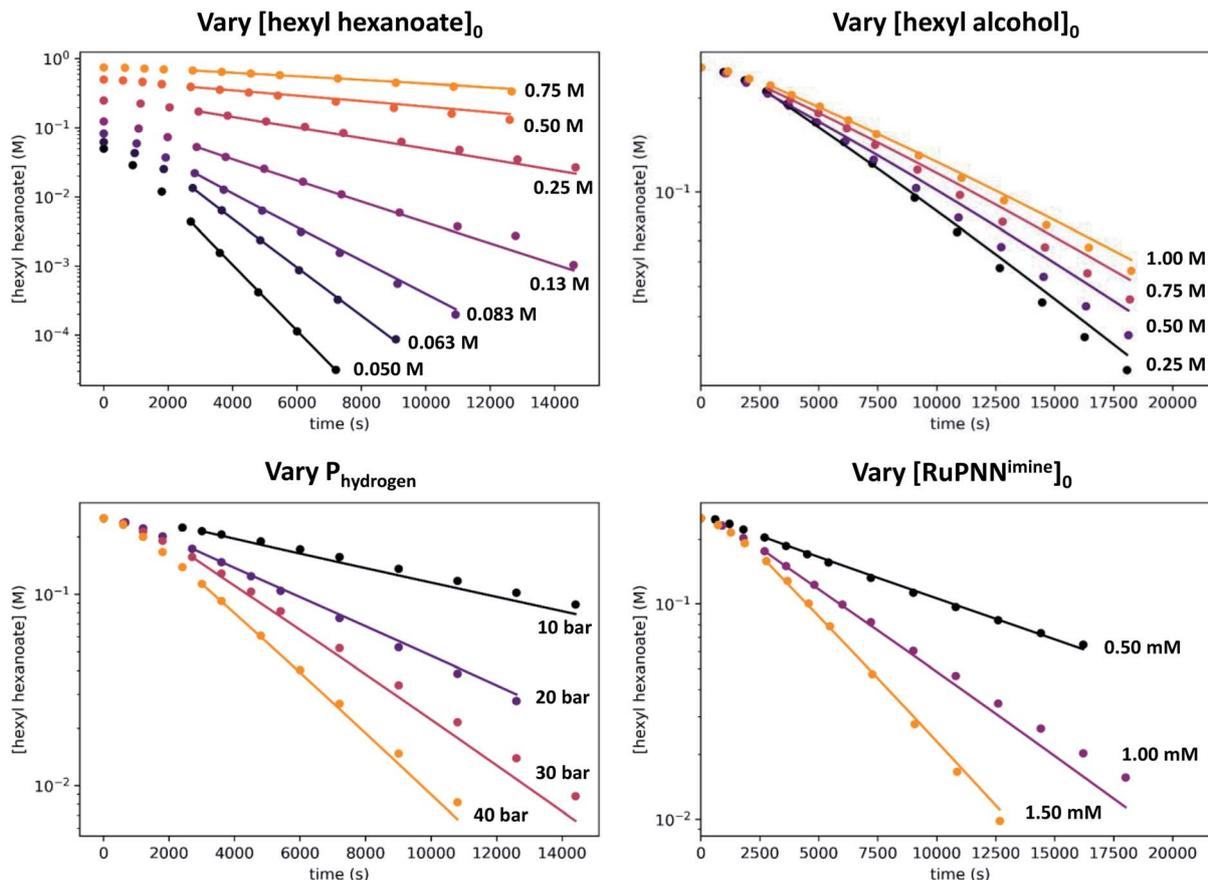
Fig. 12 Data (points) and global fit (lines) for all 18 kinetic experiments. In the standard conditions,  $[\text{hexyl hexanoate}]_0 = 0.25 \text{ M}$ ,  $[\text{hexyl alcohol}]_0 = 0 \text{ M}$ ,  $[\text{RuPNN}^{\text{imine}}]_0 = 1.00 \text{ mM}$ , and  $P_{\text{hydrogen}} = 20 \text{ bar}$ . The global fit was based on all data from 45 minutes on in each kinetic experiment. Note that the vertical axes are plotted logarithmically.
