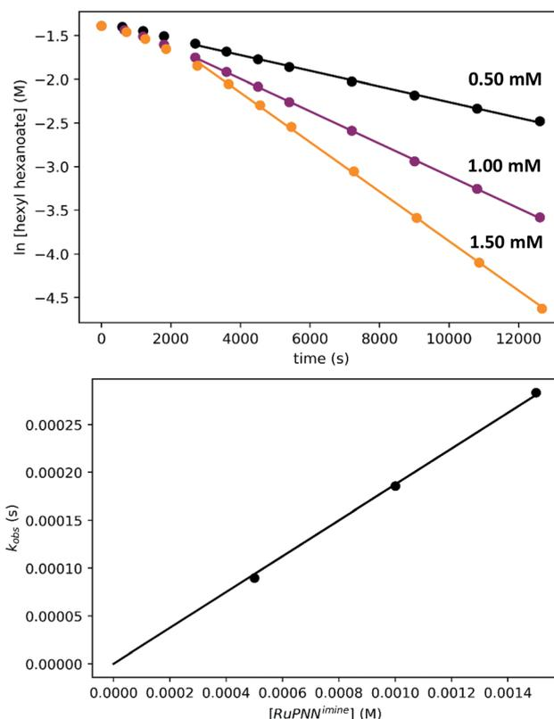
Fig. 9 Determination of the partial order in  $\text{RuPNN}^{\text{imine}}$  under the standard conditions. The top plots show the time course of ester conversion using different initial concentrations of  $\text{RuPNN}^{\text{imine}}$ , along with linear fits to the logarithm of  $[\text{ester}]$ , using data after the induction period of 45 minutes. The bottom plot shows the linear relationship between  $k_{\text{obs}}$  and  $[\text{RuPNN}^{\text{imine}}]$ .
