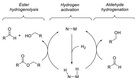
Scheme 3 Two linked catalytic cycles for ester hydrogenation.
