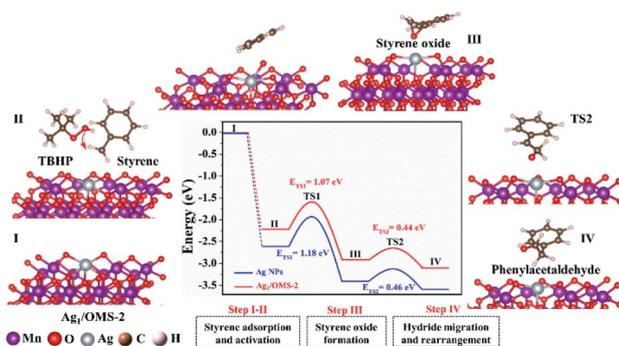
Fig. 5 DFT calculation proposed a reaction pathway for the Wacker oxidation of styrene to phenylacetaldehyde on Ag<sub>1</sub>/OMS-2, and the calculated energy profiles for Ag<sub>1</sub>/OMS-2 (red line) and Ag NPs (blue line).
