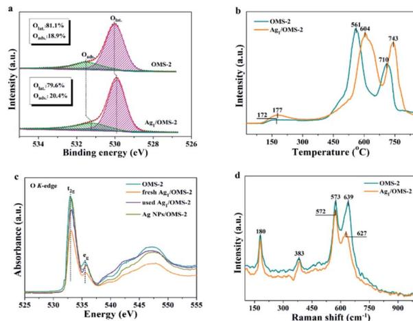
Fig. 4 (a) O 1s XPS, (b) O<sub>2</sub>-TPD, (c) O K-edge XANES, and (d) Raman profiles of OMS-2 and Ag<sub>1</sub>/OMS-2.
