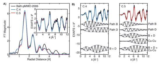
Fig. 12 (A) Fits C.4 and C.5 of Bath-pMMO-2006 as detailed in Table 4. The FT spectra were calculated over a k-range of 2–12 Å<sup>-1</sup>. (B) Selected fitted paths of fits C.4 and C.5 and summations of their signal envelopes.
