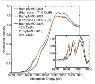
Fig. 3 Newly collected Cu PFY-XAS of Bath-pMMO-2021 compared with previously published XAS of Bath-pMMO-2006 (ref. 16) and 20Z-pMMO-2018.<sup>23</sup> The percent Cu(II) speciation is from EPR spectroscopic quantification as detailed in Table 1. Inset depicts first derivative spectra.
