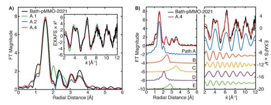
Fig. 9 (A) Selected EXAFS fits of pMMO-Bath-2021 with EXAFS parameters detailed in Table 2. The data were fit of over an R-range of 1–4 Å, and the FT-EXAFS was calculated from a k-range of 2–12 Å<sup>-1</sup>. (B) The individual fitted EXAFS paths of Fit A.4.
