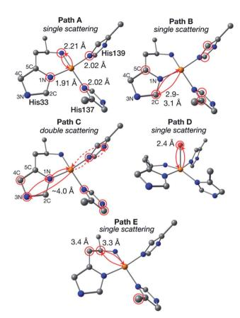
Fig. 8 Generalized EXAFS scattering paths determined for the  $\text{Cu}_{\text{B}}$  site. The calculated model is taken from ref. 17. Atom colors: Cu, orange; N, blue; C, gray; O, red; H omitted. Atoms of degenerate scattering paths are circled in red. Examples of both scattering directions of path C are shown in solid and dashed lines.
