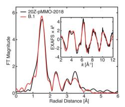
Fig. 10 Best EXAFS fitting of 20Z-pMMO-2018 as detailed in Table 3. The data were fit over an R-range of 1–4 Å, and the FT-EXAFS was calculated from a k-range of 2–12 Å<sup>-1</sup>.
