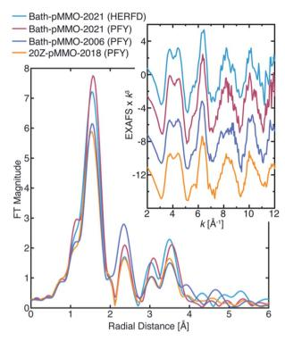
Fig. 5 FT-EXAFS of various pMMO samples collected by either the HERFD- or PFY-EXAFS technique. The **Bath-pMMO-2021** samples plotted here are of the high conc. sample set. The FT spectra were calculated from the  $k^3$ -weighted EXAFS spectra shown in the inset, over a k-range of 2–12 Å<sup>-1</sup>.
