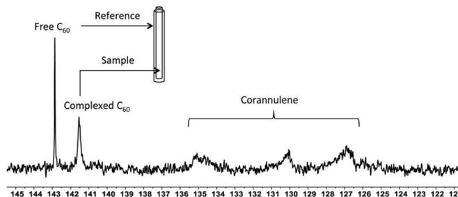
Fig. 5  $^{13}\text{C}$  NMR showing signals from the free  $C_{60}$  added as an external standard in the outer tube (reference) in deuterated tetrachloroethane and complexed  $C_{60}$  within the core of the crosslinked nanoparticle present in the inner tube (sample) also in deuterated tetrachloroethane. The internal tube diameter was 3 mm, while the external tube diameter was 5 mm.
