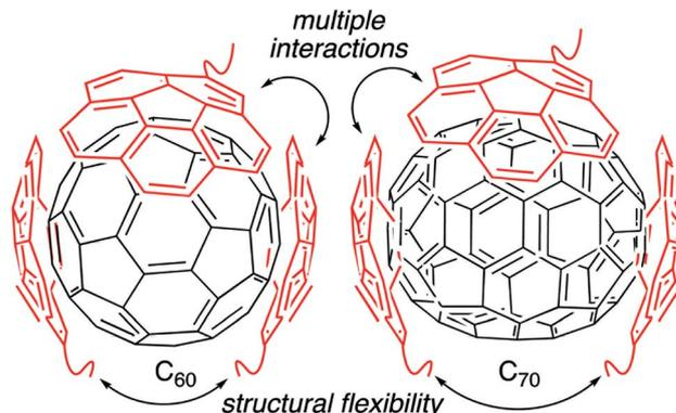
**Fig. 2** The hosting polymer block contains many corannulene units attached to the polymer backbone through a linker that can adjust upon receiving the guest molecule. These features allow accommodating different fullerene sizes in the micellar core.
