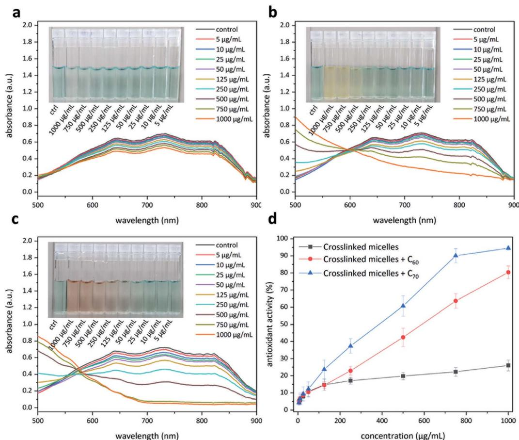
Fig. 9 Antioxidant activity of the polymer nanoparticles with and without fullerenes. Polymer nanoparticles without fullerenes (a). Polymer nanoparticles with fullerene  $\text{C}_{60}$  (b). Polymer nanoparticles with fullerene  $\text{C}_{70}$  (c). A comparison of the three systems to evaluate the amount needed to quench 50% of the free radicals in the system (d).
