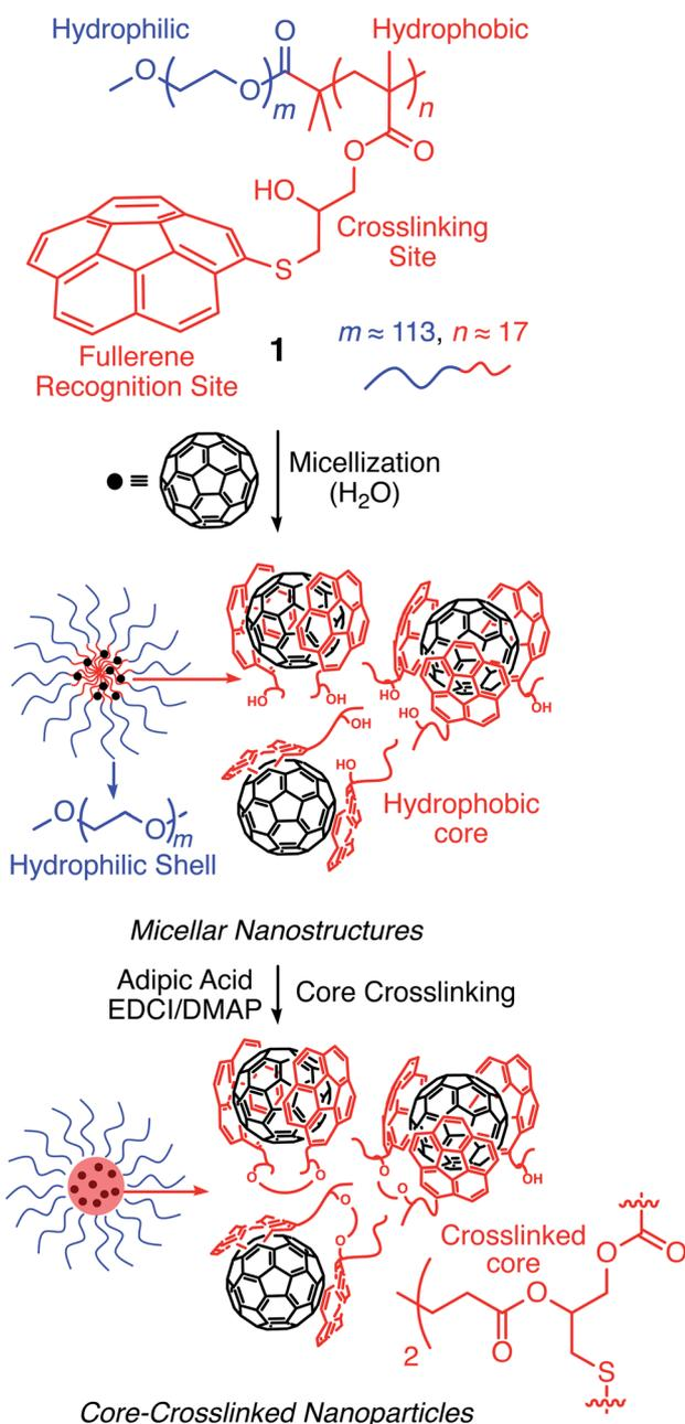
**Scheme 1** Chemical structure of host polymer **1** encoded with corannulenes and its assembly with fullerenes through ball-and-socket interactions between concave and convex aromatic surfaces to furnish micellar nanoparticles.
