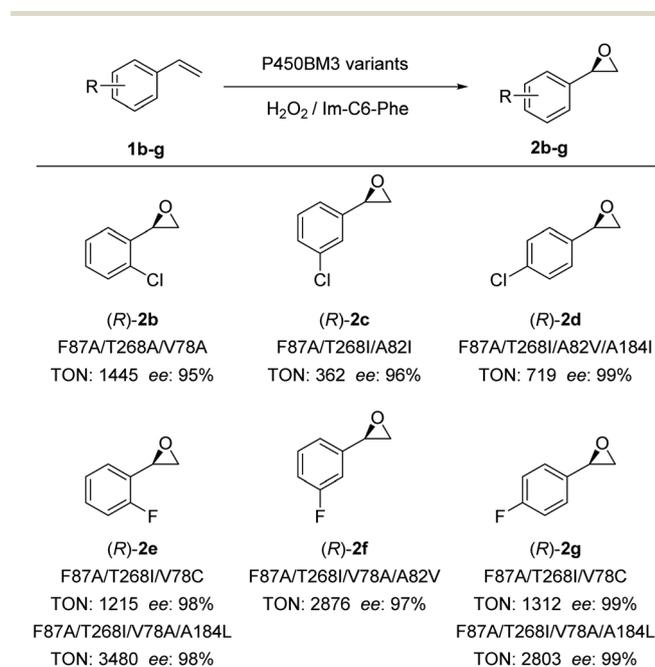
Fig. 4 Substrate scope of epoxidation reactions catalyzed by P450BM3 variants using H<sub>2</sub>O<sub>2</sub> in the presence of Im-C6-Phe. \*In some cases, trace amounts of phenyl acetaldehyde were detected by GC.
