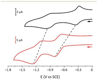
Fig. 6 Cyclic voltammograms of dumbbell 7a (black line;  $1\times10^{-4}$  M) and [3]rotaxane R6<sub>UU</sub> (red line,  $2\times10^{-4}$  M) in CH<sub>2</sub>Cl<sub>2</sub> at room temperature. A 100-fold excess of TBAPF<sub>6</sub> was employed as supporting electrolyte.
