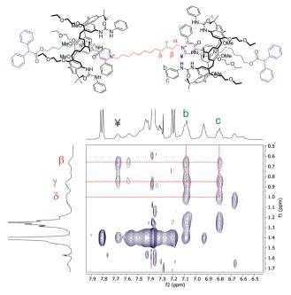
Fig. 5 Expansion of a 2D ROESY spectrum (400 MHz, CDCl<sub>3</sub>, ROESY SL = 200 ms) of R6<sub>UU</sub>. Analysis of the cross-peaks shows the spatial proximity between the protons of the internal C12 alkyl chain  $(\alpha - \delta)$  and those of the phenylurea groups (b and c) present at the upper rim of the calix[6]arene macrocycles (for the full spectrum, see ESI†).
