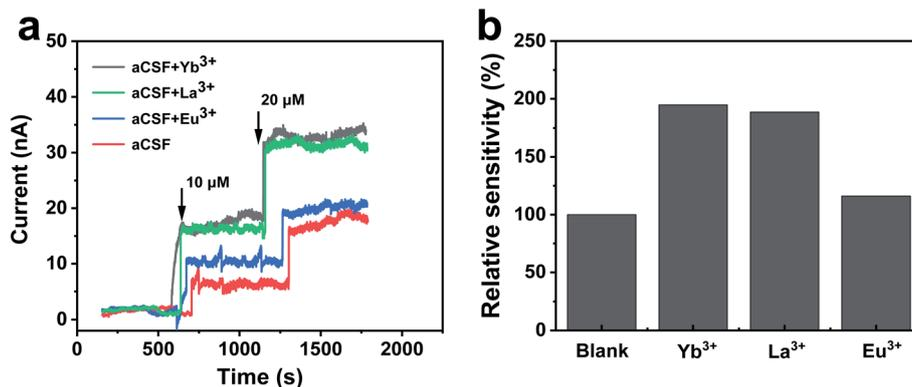
Fig. 2 Effect of REEs on bioelectrocatalytic performance of NAD<sup>+</sup>-dependent GDH. (a) Amperometric current responses of the GDH-based biosensor toward titrations of 10 and 20 μM glutamate at 0.0 V vs. Ag/AgCl in aCSF containing 2 mM NAD<sup>+</sup> in the absence or presence of 16 μM Yb<sup>3+</sup>, La<sup>3+</sup> or Eu<sup>3+</sup>. (b) Relative sensitivity of the GDH-based glutamate biosensor.
