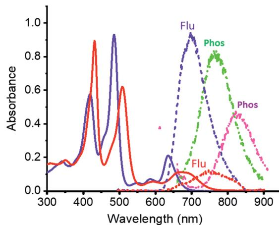
Fig. 2 Absorption (solid line), fluorescence (short dash) and phosphorescence (dot dot dash, at 77 K) spectra of **ZnP-SQ** in dichlorobenzene (DCB) in the absence (purple) and presence of F<sup>−</sup> (red for fluorescence and green (**ZnP-SQ**) and magenta (F<sup>−</sup>:**ZnP-SQ**) for phosphorescence).  $\lambda_{EX} = 485$  nm.
