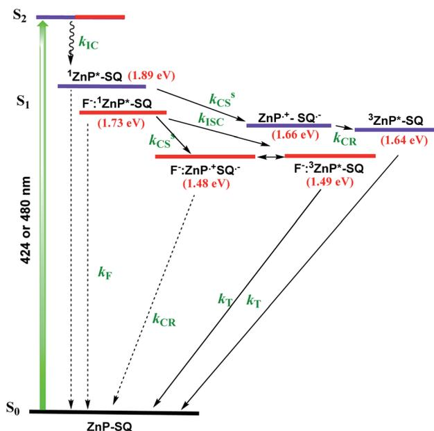
Fig. 4 Energy level diagram depicting excited state charge separation and recombination upon Soret band excitation in **ZnP-SQ** (purple) and  $F^-$ :**ZnP-SQ** (red). Abbreviations: F = fluorescence, IC = internal conversion, ISC = intersystem crossing, CS = charge separation, CR = charge recombination, S = singlet state and T = triplet state. Solid arrow = major path, dashed arrow = minor path.
