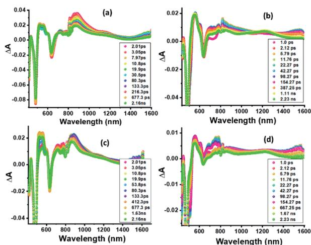
Fig. 5 fs-TA spectra at the indicated delay times of (a and c) **ZnP-SQ** and (b and d) **F<sup>-</sup>:ZnP-SQ** at the excitation wavelength of 424 (a and b) and 480 nm (c and d) in DCB.
