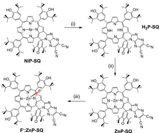
Scheme 1 Transformation of **NiP-SQ** to F<sup>−</sup>:**ZnP-SQ**. (i) c. H<sub>2</sub>SO<sub>4</sub>. (ii) Zinc acetate/CHCl<sub>3</sub>/CH<sub>3</sub>OH. (iii) Teta-*n*-butylammonium fluoride.
