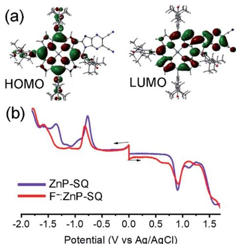
Fig. 3 (a) HOMO and LUMO structures of **ZnP-SQ** on B3LYP/6-31G\* optimized structure. (b) DPV of **ZnP-SQ** (purple) and  $F^-$ :**ZnP-SQ** (red) in DCB containing 0.1 M (TBA)ClO<sub>4</sub>. Scan rate = 5 mV s<sup>-1</sup>, pulse width = 0.25 s, pulse height = 0.025 V.
