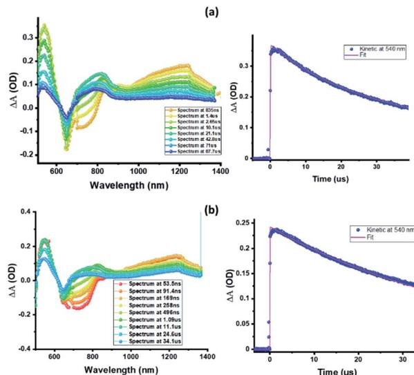
Fig. 6 Nanosecond transient absorption spectra at the indicated delay times of (a) **ZnP-SQ** and (b) **F<sup>-</sup>:ZnP-SQ** at the excitation wavelength of 480 nm in DCB.
