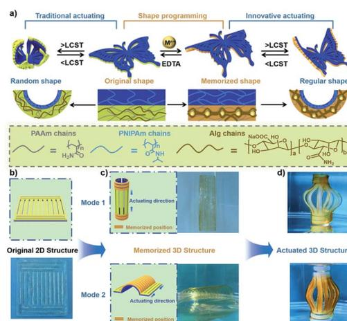
Fig. 10 (a) Schematic illustration of the traditional deformation process in programmable shape deformation generated by the combination of shape memory and actuation behavior. (b) Schematic illustration of the bilayer structure and the mechanism of shape memory and the actuation process. (c and d) Programmable deformation of a 2D sheet into a 3D lantern shape by the assistance of kirigami. Scale bars: 1 cm. Reproduced with permission from ref. 88. Copyright 2020 Wiley-VCH.
