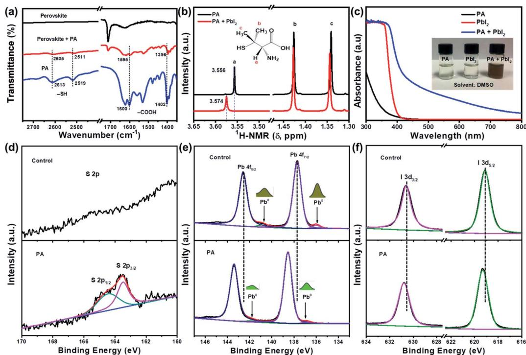
Fig. 1 (a) FTIR spectra of PA and perovskite films without and with PA. (b)  $^1\text{H-NMR}$  spectra of PA and PA containing  $\text{PbI}_2$  solutions. (c) UV-vis absorption spectra of  $\text{PbI}_2$  solutions without and with PA (inset: photographs of the corresponding solution). High resolution XPS spectra of S 2p (d), Pb 4f (e) and I 3d (f) for the perovskite films without and with PA, respectively.
