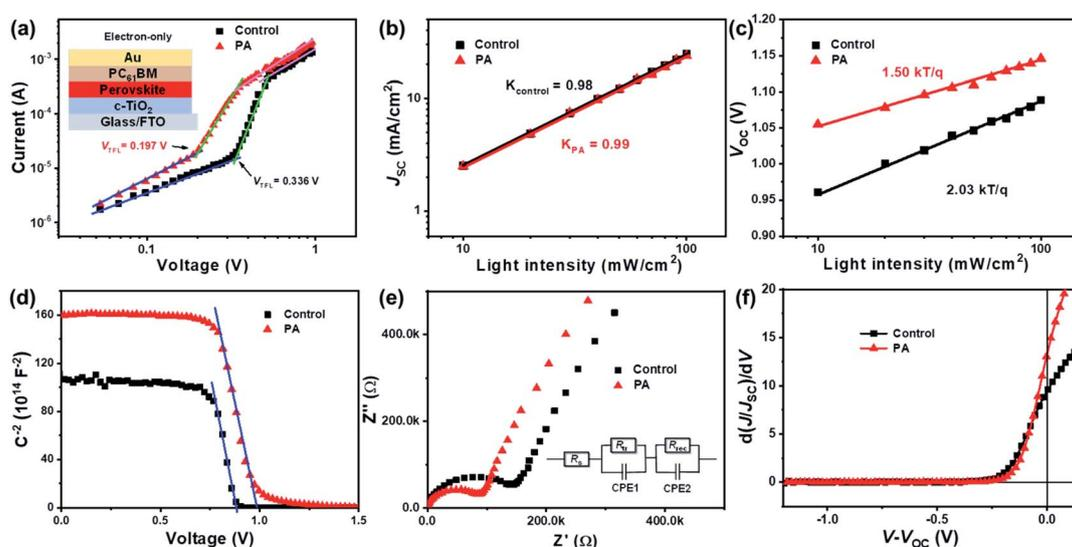
Fig. 5 (a) Dark  $I$ - $V$  curves for the electron-only devices based on the control and PA containing perovskite. (b)  $J_{SC}$  vs. light intensity and (c)  $V_{OC}$  vs. light intensity for the devices without and with PA. (d) Mott-Schottky fitting to the capacitance-voltage ( $C^{-2}$ - $V$ ) plots and (e) EIS of PSCs based on control and PA containing perovskite film. (f) The slopes of the normalized  $J$ - $V$  curves at each voltage for the champion control and PA containing devices.
