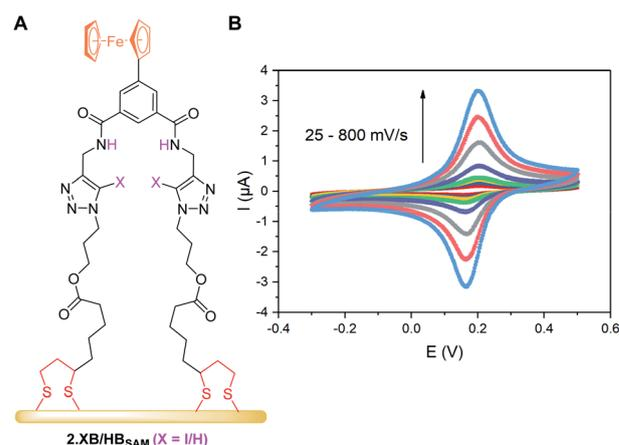
**Fig. 4** (A) Schematic representation of **2.XB/HB**<sub>SAM</sub> on a gold electrode. (B) CVs at varying scan rate of **2.HB**<sub>SAM</sub> in ACN, 100 mM TBAClO<sub>4</sub>. The associated anodic and cathodic peak currents as a function of the square-root of the scan rate are shown in Fig. S25.†
