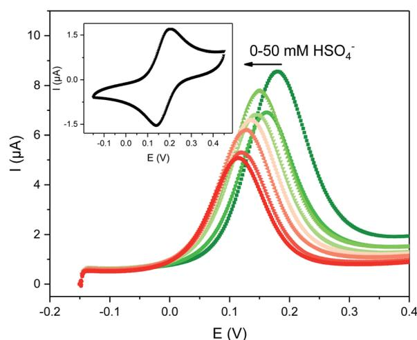
Fig. 2 Evolution of the square-wave voltammograms (SWVs) of 0.1 mM **1.XB** in ACN, 100 mM TBAClO<sub>4</sub> upon titration with TBAHSO<sub>4</sub>. The inset shows the CV of this receptor at a scan rate of 100 mV s<sup>-1</sup>.
