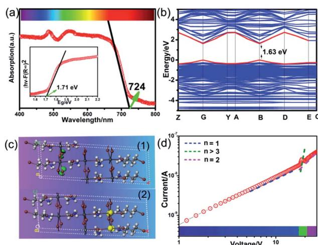
Fig. 2 (a) UV-Vis absorption spectrum for **IMP**. Inset: calculated bandgap of **IMP**. (b) Theoretically calculated band structure of **IMP**. (c) The calculated charge density isosurfaces for HOMO (1) and LUMO (2) orbitals. (d) Logarithmic  $I$ - $V$  characteristics of **IMP** based on the space charge limited current method.
