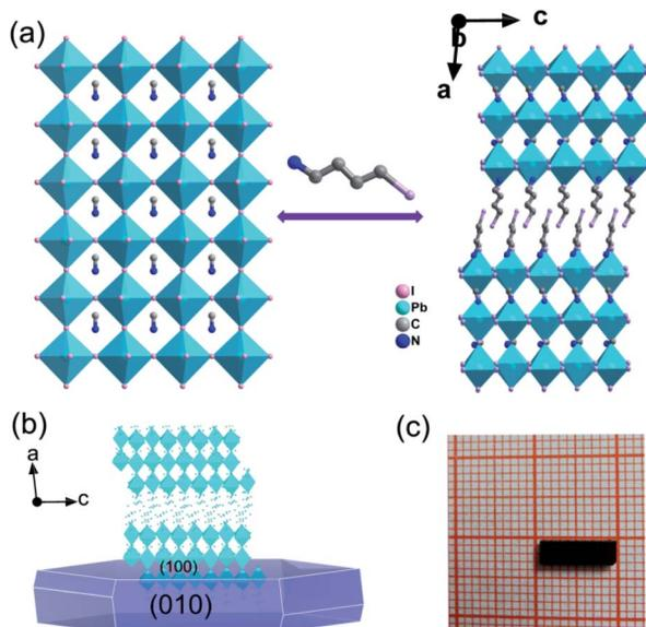
Fig. 1 (a) Trimming three-dimensional  $\text{CH}_3\text{NH}_3\text{PbI}_3$  to design a 2D structure of **IMP** viewed along the  $b$ -axis. (b) Typical growth morphology for crystals of **IMP**. (c) Solution-grown bulk crystal of **IMP** with dimensions of  $9.0 \times 3.0 \times 1.5 \text{ mm}^3$ .
