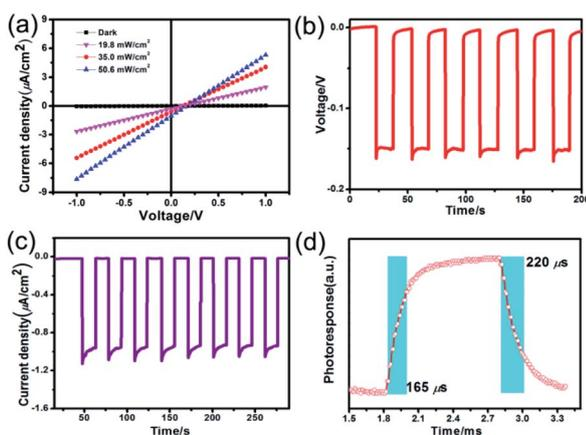
Fig. 3 (a) Current-voltage characteristics along polarization directions of **IMP** with different incident power (along a 637 nm laser). (b) Reproducible bulk photovoltaic on/off switching. (c) Reproducible photocurrent on/off switching at zero bias. (d) The rise and fall of the photocurrent at zero bias.
