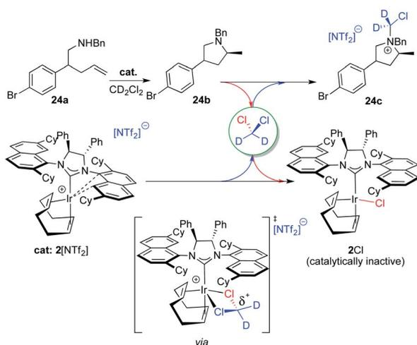
Fig. 8 Proposed deactivation pathway for 2[NTf<sub>2</sub>], forming **24c** and 2Cl *via* the intermediate shown.
