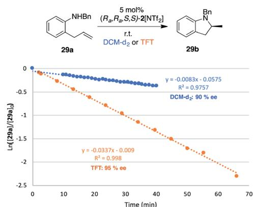
Fig. 10 Plot of Ln([29a]<sub>t</sub>/[29a]<sub>0</sub>) vs. time of substrate **29a** to indoline **29b** using (*R*<sub>a</sub>,*R*<sub>a</sub>,*S*,*S*)-2[NTf<sub>2</sub>] at 5 mol%. Reactions conducted in DCM-d<sub>2</sub> or TFT (0.5 mL), [29a] = 0.6 M, [Ir] = 0.03 M. Conversion monitored using <sup>1</sup>H NMR.
