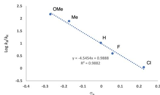
Fig. 13 Hammett plot for HA of anilines **29a–33a** with 2[NTf<sub>2</sub>] (TFT, 25 °C). Concentrations: [**29a–33a**] = 0.6 M and [Ir] = 0.03 M.
