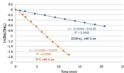
Fig. 9 Plot of  $\ln([5a]/[5a]_0)$  vs. time of model substrate **5a** to pyrrolidine **5b** vs. time (min) using (*R*<sub>a</sub>,*R*<sub>a</sub>,*S*,*S*)-2[NTf<sub>2</sub>] at 0.5 mol%. Reactions conducted in DCM-d<sub>2</sub> or TFT (0.5 mL), [5a] = 0.6 M, [Ir] = 0.003 M. Conversion monitored using <sup>1</sup>H NMR.
