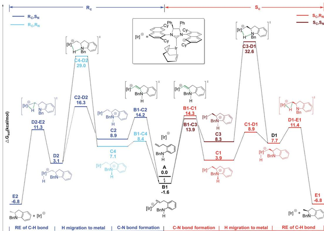
Scheme 2 Energy profile for C=C activation pathway for HA reaction of indoline **29a** in the presence of **2**. Free energies in kcal mol<sup>-1</sup>.
