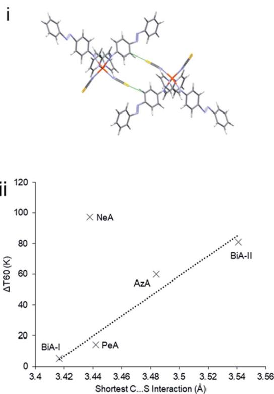
Fig. 1 (i) S···H–C interactions in  $[\text{Fe}(\text{PM-AzA})_2(\text{NCS})_2]$ . (ii) Relationship between the S···C interaction distance and SCO transition abruptness ( $\Delta T_{60}$ ) in the  $[\text{Fe}(\text{PM-L})_2(\text{NCS})_2]$  complexes of Scheme 1. The S···C distance is measured in the HS form in each case. BiA-I and BiA-II correspond to different polymorphs. The values plotted are available in Table S4.†
