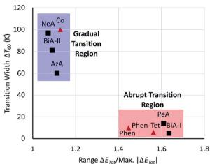
Fig. 8 Transition width ( $\Delta T_{60}$ ) against range  $\Delta E_{Tot}/\text{max}$  | $\Delta E_{Tot}|$  for Fe(PM-L)<sub>2</sub>(NCS)<sub>2</sub> SCO complexes (black squares) and other SCO complexes (red trianges). Range  $\Delta E_{Tot}$  is defined as [most +ve  $\Delta E_{Tot}$ ] – Imost –ve  $\Delta E_{Tot}$ ].
