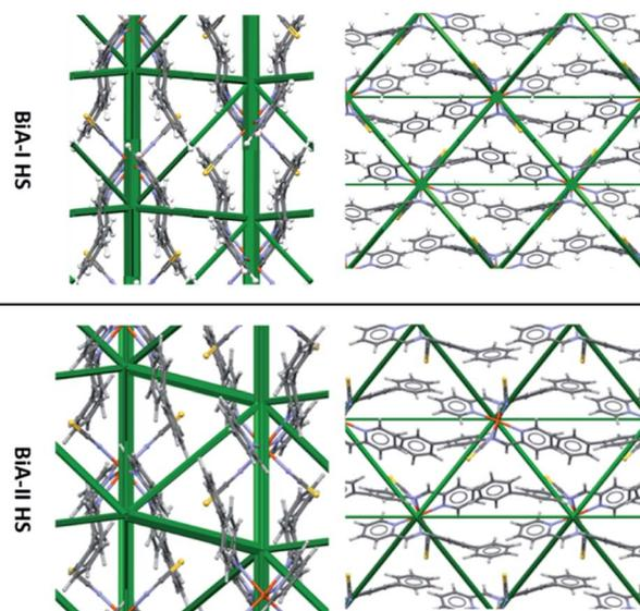
Fig. 3 Comparison of HS energy frameworks for  $[\text{Fe}(\text{PM-BiA})_2(\text{NCS})_2]$  polymorphs I and II viewed along the *a* axis (left) and *c* axis (right). A comparison of the LS forms is shown in Fig. S6.†
