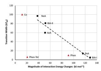
Fig. 6 The transition abruptness ( $\Delta T_{60}$  in K) plotted against the sum of the of absolute total interaction energy changes for [Fe(PM-L)<sub>2</sub>(NCS)<sub>2</sub>] SCO complexes (black squares) and three other SCO complexes (red trianges, see text). The equation of the fitted line is y = -0.9428x + 124.04.
