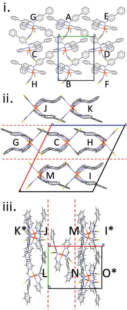
Fig. 2 Stacking of layers in  $[\text{Fe}(\text{PM-BiA})_2(\text{NCS})_2]$  polymorph-II. Contacts to a central reference molecule are labelled A, B... layers (separated by red hashed lines), are viewed along the *a* (i), *b* (ii) and *c* (iii) axes, respectively. The reference molecule overlaps C in projection in (ii); where molecules are in background, labels are denoted with \*.
