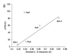
Fig. 1 (i) S···H–C interactions in [Fe(PM-AzA)<sub>2</sub>(NCS)<sub>2</sub>]. (ii) Relationship between the S···C interaction distance and SCO transition abruptness ( $\Delta T_{60}$ ) in the [Fe(PM-L)<sub>2</sub>(NCS)<sub>2</sub>] complexes of Scheme 1. The S···C distance is measured in the HS form in each case. BiA-I and BiA-II correspond to different polymorphs. The values plotted are available in Table S4.†
