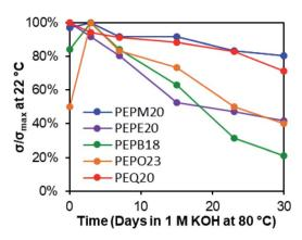
Fig. 2 Membrane hydroxide conductivity stability under 1 M KOH $_{\rm aq}$  at 80  $^{\circ}$ C in PP vials for 30 days.
