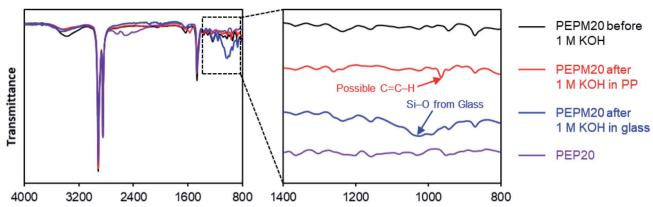
Fig. 3 FT-IR spectra of membranes before and after alkaline treatment to study degradation mechanisms.
