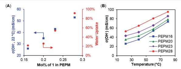
Fig. 1 (A) Membrane hydroxide conductivity and water uptake of PEPMs with different ionic contents. (B) Membrane hydroxide conductivities of PEPMs under different temperatures.
