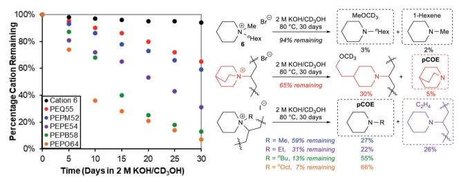
Fig. 4 Alkaline stability evaluation of model compound  $\bf 6$  and oligomers under 2 M KOH/CD<sub>3</sub>OH conditions at 80 °C for 30 days: degradation kinetics by  $^{1}$ H NMR analysis (left) and byproduct assignment (right).
