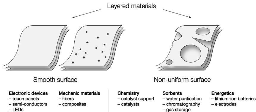
Fig. 1 A few representative areas of application of different smooth materials and materials with defects. Stars represent uniformly distributed point defects.
