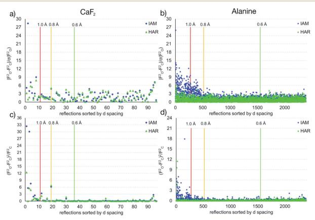
Fig. 7 Differences of observed and calculated structure factors versus resolution for CaF2 and L-Ala for the IAM and the HAR models.
