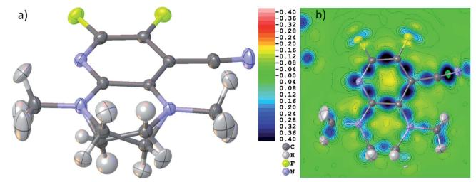
Fig. 5 (a) Final HAR geometry after disorder treatment of THPP. (b) Dynamic deformation density distribution in the main molecular plane of the molecule. Color scale legend in eÅ<sup>-3</sup>. Atomic anisotropic and isotropic displacement parameters at 80% probability level.
