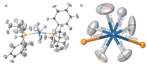
Fig. 9 (a) HAR-refined molecular structure of  $OsH_6(PC_{12}H_{19})_2$  with the PBE-DKH2/x2c-TZVPP model at full resolution. (b) Coordination geometry of the Os atom with the freely refined distances to the six nearest hydrogen and two nearest phosphorus atoms. All displacement parameters are displayed at 80% probability level.
