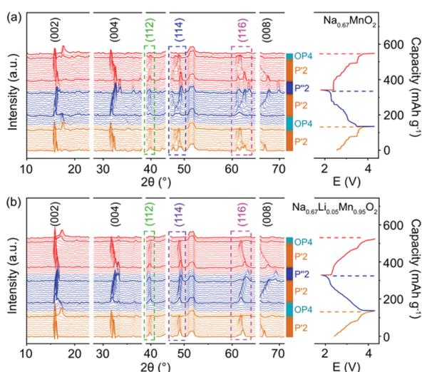
Fig. 2 *In situ* XRD patterns collected in the first cycle and second charge of (a) P'2-Na<sub>0.67</sub>MnO<sub>2</sub> and (b) P'2-Na<sub>0.67</sub>Li<sub>0.05</sub>Mn<sub>0.95</sub>O<sub>2</sub>.
