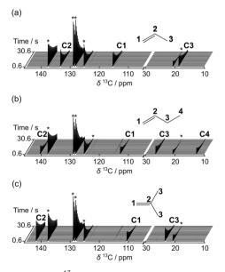
Fig. 2 Hyperpolarized  $^{13}$ C NMR spectra of (a) propene, (b) 1-butene, and (c) isobutene. Every 4th acquired spectrum is shown from data sets with an acquisition delay of 500 ms. Each spectrum was measured following an excitation pulse with a flip angle of  $10.2^{\circ}$ . Labels C1–C4 indicate signals from the carbon atoms indicated in the structural drawings. Signals from toluene included in the matrix for DNP polarization are designated with  $^{*}$ .
