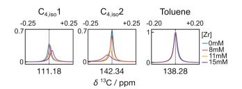
Fig. 5 The C1 and C2 signals of isobutene ( $C_{4,iso}$ 1 and  $C_{4,iso}$ 2, respectively) from the polymerization reactions, as well as in the absence of a reaction. Signals are from spectra measured at t=0.61 s. The toluene signal from the quaternary carbon (138.28 ppm) was used for intensity normalization in each spectrum.
