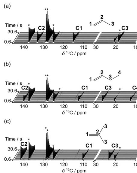
Fig. 2 Hyperpolarized <sup>13</sup>C NMR spectra of (a) propene, (b) 1-butene, and (c) isobutene. Every 4th acquired spectrum is shown from data sets with an acquisition delay of 500 ms. Each spectrum was measured following an excitation pulse with a flip angle of 10.2°. Labels C1–C4 indicate signals from the carbon atoms indicated in the structural drawings. Signals from toluene included in the matrix for DNP polarization are designated with \*.
