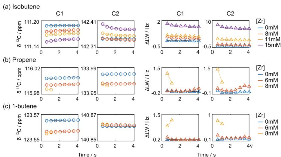
Fig. 6 Chemical shifts and line widths of C1 and C2 monomer signals from (a) isobutene (b) propene and (c) 1-butene polymerization reactions measured over time. Plots in the left two columns display the changes in chemical shift (circles), and those in the right two columns show the line width changes (triangles). For propene and 1-butene polymerizations with  $[Zr] = 8$  mM, two data points are shown, as the monomer signal intensities are at the noise level at subsequent time points.
