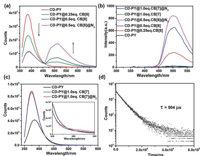
Fig. 2 The prompt photoluminescence (a and c) (inset of (c): the enlarged luminescence peak at 510 nm) and gated (0.1 ms) spectra (b) of CD-PY with or without CB[7,8] and  $N_2$  in aqueous solution. (d) Decay curve of CD-PY@CB[8] (1 : 0.5) aqueous solution at 510 nm ( $[CD-PY] = 0.5 \text{ mM}$ ,<sup>44,54,60</sup> Ex = 340 nm, 298 K).
