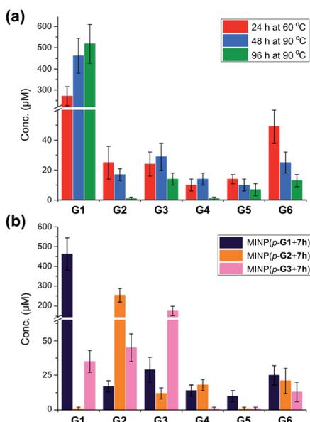
**Fig. 1** (a) Product distributions for the hydrolysis of 100 μM maltohexaose (G6) under different conditions for the hydrolysis of 20 μM MINP(*p*-G1 + 7h) in 10 mM MES buffer (pH 6). (b) Product distributions for the hydrolysis of 0.1 mM maltohexaose (G6) using different MINPs (20 μM) in 10 mM MES buffer (pH 6) at 90 °C for 48 h. See Table S4† for the exact numbers.
