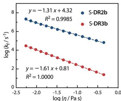
Fig. 9 Dependence of the solvent thermal fluctuation rate constant  $\log k_f$  calculated by eqn (2) on the viscosity of GTA.  $k_{\text{Ac}}$  and  $k_{\text{GTA}}$  were calculated from the Eyring plot.
