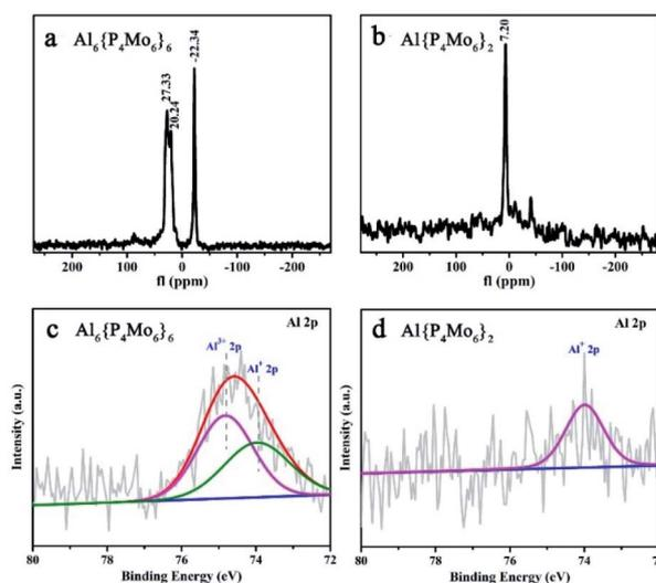
Fig. 3 (a and b)  $^{27}\text{Al}$  NMR spectra of solid  $\text{Al}_6\{\text{P}_4\text{Mo}_6\}_6$  and  $\text{Al}\{\text{P}_4\text{Mo}_6\}_2$ ; (c and d) XPS spectra of Al in  $\text{Al}_6\{\text{P}_4\text{Mo}_6\}_6$  and  $\text{Al}\{\text{P}_4\text{Mo}_6\}_2$ .
