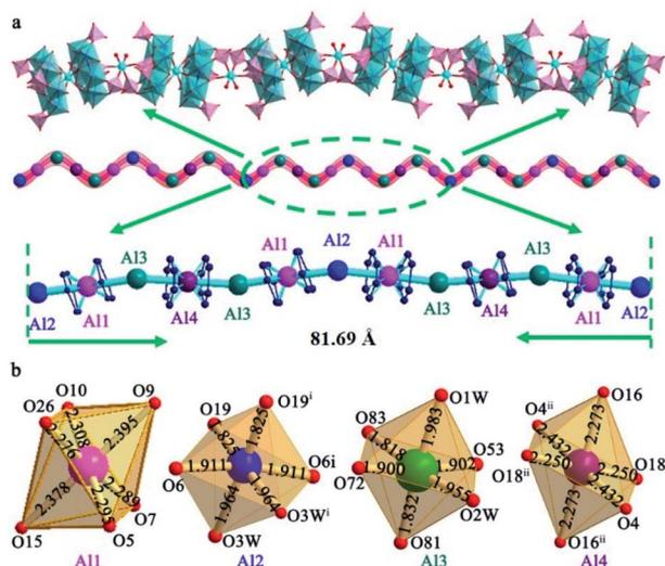
Fig. 2 (a) One-dimensional (1D) inorganic structure in  $\text{Al}_6\{\text{P}_4\text{Mo}_6\}_6$  with a length of repeating units of 81.69 Å, consisting of twelve Al-containing fragments ( $\{-\text{Al}_2-\text{Al}_1-\text{Al}_3-\text{Al}_4-\text{Al}_3-\text{Al}_1-\text{Al}_2-\text{Al}_1-\text{Al}_3-\text{Al}_4-\text{Al}_3-\text{Al}_1-\}$ ). (b) Four kinds of coordination environments of  $\{\text{AlO}_6\}$  octahedra, respectively ( $i = 1 - x, y, 0.5 - z; ii = 0.5 - x, 1.5 - y, 1 - z$ ).
