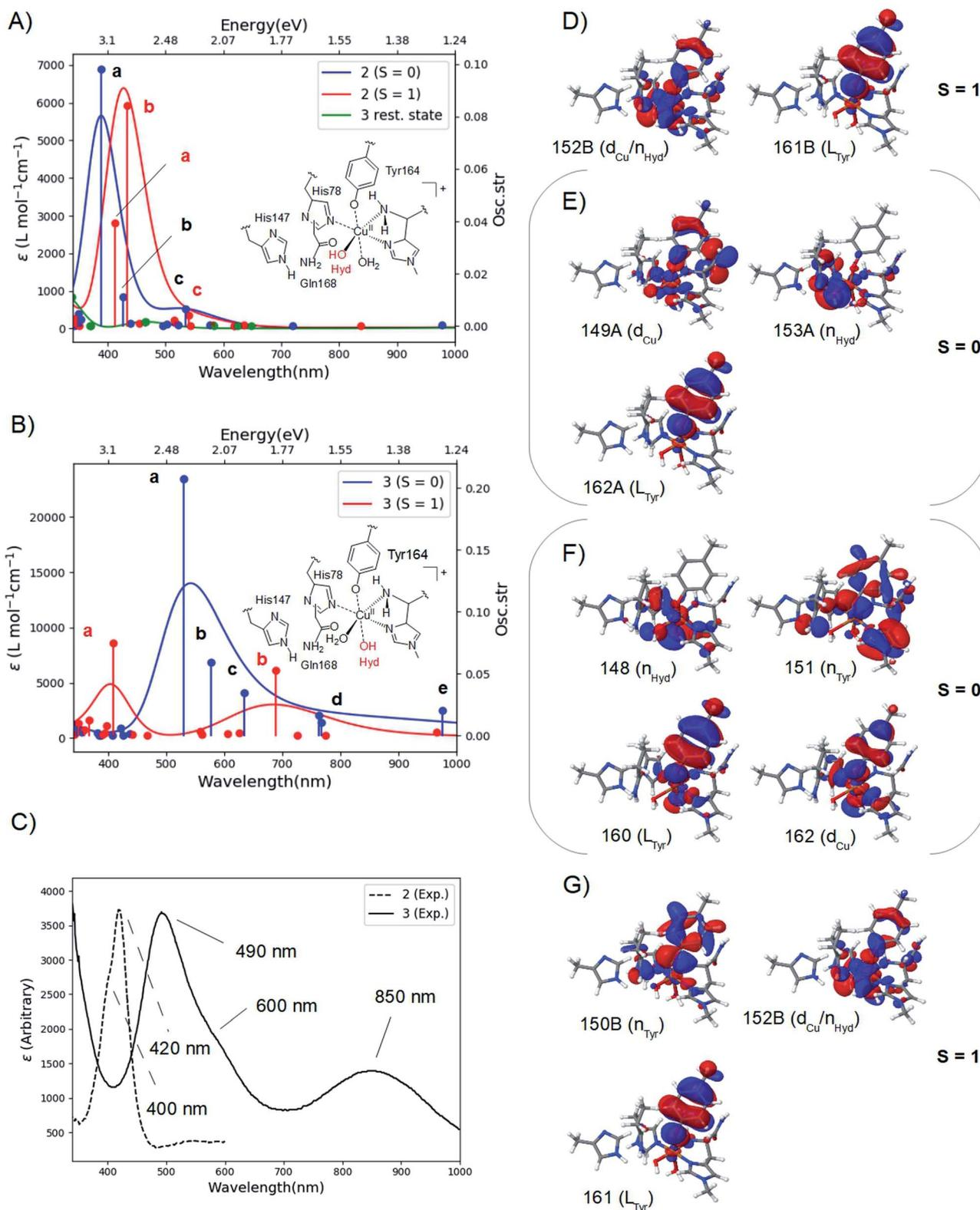
Fig. 2 Calculated spectra for the resting state, 2 (A) and 3 (B) with CAM-B3LYP/def2-TZVPP from TPSS/def2-SV(P) QM/MM structures. The experimental spectra<sup>38,39</sup> are shown in (C), with the intensity of 2 scaled. Intense transitions are labelled a–e. Selected, involved orbitals are shown for 2 in (D) and (E) and for 3 in (F) and (G). The orbitals are labeled after their main character and by their numbers (see the ESI† for further details).
