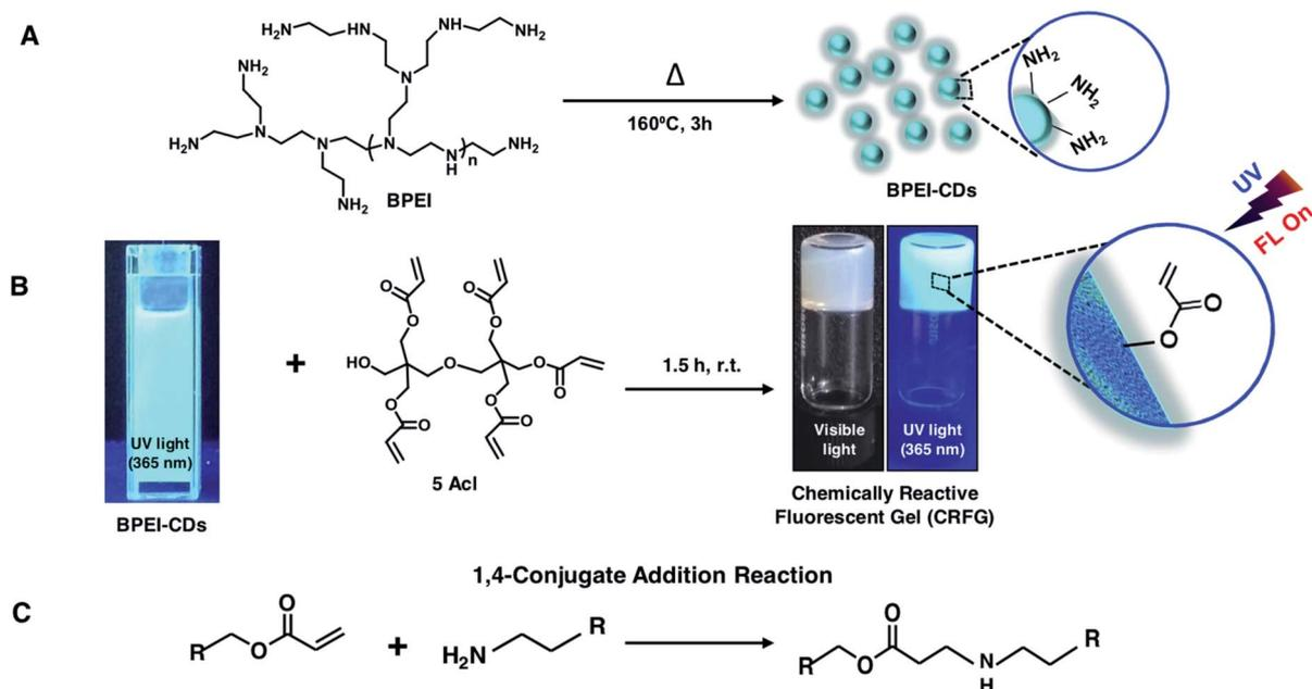
**Scheme 1** (A) A schematic diagram depicting the synthesis of carbon dots from BPEI via a hydrothermal process. (B) The formation of a chemically reactive and fluorescent gel (CRFG) through a facile 1,4-conjugate addition reaction (C) between the amines of BPEI-CDs and acrylates of 5Acl under ambient conditions.
