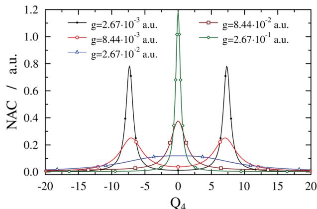
Fig. 5 Nonadiabatic coupling (1D( $v_4$ ) model) as a function of  $Q_4$  for formaldehyde in a cavity of  $\omega_c = 27\,653.3\text{ cm}^{-1}$  with different coupling strength values  $g$ . With growing coupling strength, the bimodal structure of the nonadiabatic coupling turns into a single maximum following the structure of the avoided crossings of the adiabatic potentials shown in Fig. 4.
