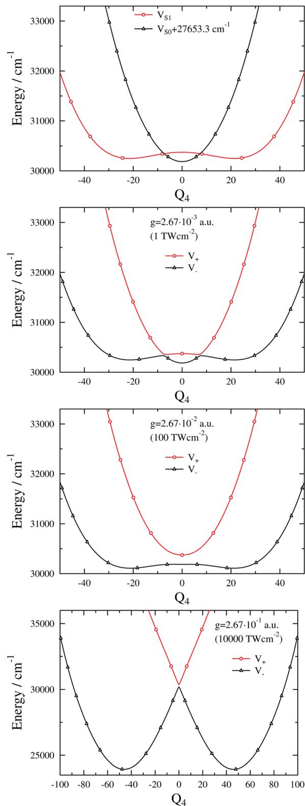
Fig. 4 1D( $v_4$ ) diabatic (uppermost panel) and adiabatic potential curves ( $V_+$  and  $V_-$ ) with a cavity wavenumber of  $\omega_c = 27\,653.3\text{ cm}^{-1}$  for different coupling strength values. Note that the range of the energy axis in the last panel ( $g = 2.67 \times 10^{-1}\text{ a.u.}$ ) differs from those of the other three panels.
