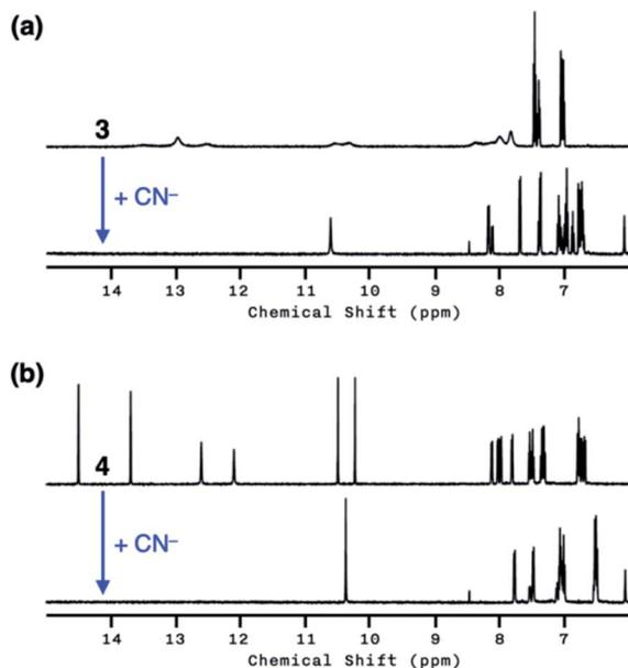
Fig. 8 (a)  $^1\text{H}$  NMR spectra of **3** (4.0 mM) in  $\text{DMSO}-d_6$  prior to (top) and after (bottom) the addition of  $\text{NaCN}$  (10 equiv.). (b)  $^1\text{H}$  NMR spectra of **4** (4.0 mM) in  $\text{DMSO}-d_6$  prior to (top) and after (bottom) the addition of  $\text{NaCN}$  (10 equiv.).  $T = 298\text{ K}$ .
