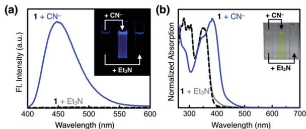
Fig. 10 (a) Emission ( $\lambda_{\text{exc}} = 343$  nm) and (b) absorption spectra of **1** (0.100 mM, black dashed lines), and spectral changes induced by treatment with NaCN (25 equiv., blue lines) and with  $\text{Et}_3\text{N}$  (25 equiv., gray lines) in DMSO at  $T = 298$  K. Inset: photographic images of (a) fluorescence response (under a 365 nm UV lamp) and (b) color change.
