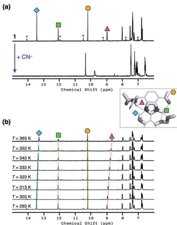
Fig. 11 (a)  $^1\text{H}$  NMR spectra of **1** (4.0 mM) prior to (top) and after (bottom) the addition of NaCN (10 equiv.) in  $\text{DMSO}-d_6$  at  $T = 298$  K. Asterisks indicate the resonances of the minor tautomer which is less than 10% based on the peak integration values. (b) Variable-temperature  $^1\text{H}$  NMR spectra of **1** (4.0 mM) in  $\text{DMSO}-d_6$  at  $T = 293$ – $363$  K.
