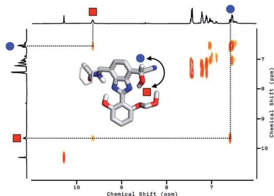
Fig. 12 Partial 2D-COSY contour plot of **1** (4.0 mM) treated with NaCN (10 equiv.) in  $\text{DMSO}-d_6$  at  $T = 298$  K. The corresponding 1D NMR spectrum is shown along the ordinate. Inset: DFT (B3LYP-D3/6-31G(d,p)) energy-minimized structure of the cyanohydrin adduct of **1**.
