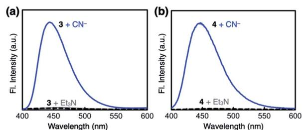
**Fig. 7** Emission spectra ( $\lambda_{\text{exc}} = 343 \text{ nm}$ ) of (a) 3 (0.100 mM) prior to (black dashed lines) and after treatment with NaCN (25 equiv., blue line) or  $\text{Et}_3\text{N}$  (25 equiv., gray line), and (b) 4 (0.100 mM) prior to (black dashed lines) and after treatment with NaCN (25 equiv., blue line) or  $\text{Et}_3\text{N}$  (25 equiv., gray line) in DMSO at  $T = 298 \text{ K}$ .
