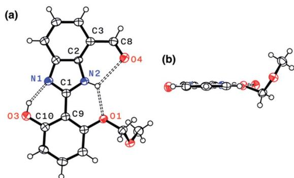
**Fig. 6** X-ray structure of 4 as ORTEP diagrams with thermal ellipsoids at the 50% probability level: (a) face-on and (b) edge-on views. Selected interatomic distances (Å) of the hydrogen bonds (dashed lines):  $\text{N1}\cdots\text{O3}$ , 2.568(3);  $\text{N2}\cdots\text{O1}$ , 2.634(4);  $\text{N2}\cdots\text{O4}$ , 2.901(3).
