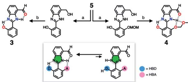
**Scheme 3** Construction of a hydrogen bonding network to shift the tautomer equilibrium. (a) Aldehyde,  $\text{Na}_2\text{S}_2\text{O}_5$ , EtOH,  $\text{H}_2\text{O}$ ,  $\Delta$ . (b)  $\text{MnO}_2$ , MeCN/ $\text{CH}_2\text{Cl}_2$ , r.t.
