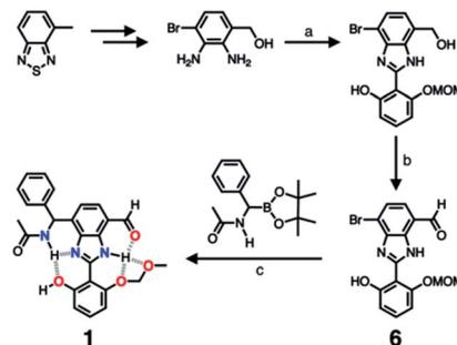
Scheme 4 Synthetic route to **1**. (a) Aldehyde,  $\text{Na}_2\text{S}_2\text{O}_5$ ,  $\text{EtOH}/\text{H}_2\text{O}$ ,  $\Delta$ . (b)  $\text{MnO}_2$ ,  $\text{MeCN}/\text{CH}_2\text{Cl}_2$ , r.t. (c)  $\text{Pd}_2(\text{dba})_3$ ,  $\text{P}(\text{tBu})_3$ ,  $\text{HBF}_4$ ,  $\text{KF}$ , dioxane/ $\text{H}_2\text{O}$ ,  $\Delta$ .
