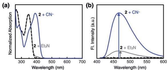
Fig. 4 (a) Absorption and (b) emission spectra ( $\lambda_{\text{exc}} = 400$  nm) of **2** (0.100 mM) prior to (black dashed lines) and after treatment with NaCN (25 equiv., blue lines) or  $\text{Et}_3\text{N}$  (25 equiv., gray lines) in DMSO at  $T = 298$  K.
