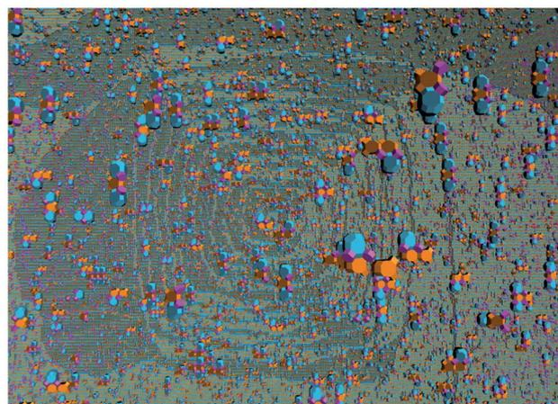
**Fig. 17** Point defect clusters within the interior of STA-7 crystals that form spontaneously during crystal growth. Orange cages are *t-sav* tiles, blue cages *t-fup* and purple cages *t-hpr*. The background is the internal side of the far exterior of the crystal that shows an impression of the (100) screw dislocation.
