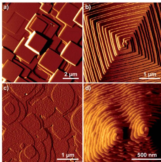
**Fig. 4** AFM micrographs of MOF-5 and ZIF-8 crystal surfaces. Well-defined square shapes can be seen for MOF-5 terraces grown by the birth-and-spread mechanism (a) along with those grown through screw dislocations (b). Well-defined terrace shapes can also be seen for ZIF-8, with rounded rhombus terraces grown through birth-and-spread mechanism (c) and round terraces grown through spiral growth caused by screw dislocations (d).
