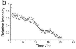
(a) Intensity contour plot showing the time-dependence of the in situ <sup>31</sup>P NMR spectrum (recorded without <sup>1</sup>H decoupling) at 60 °C, representing the liquid-state <sup>31</sup>P NMR signal. (b) Intensity vs. time plot for the liquid-state <sup>31</sup>P NMR signal.
