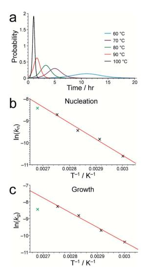
Fig. 4 (a) The nucleation probability distribution for MFM-500(Ni) formation, obtained by fitting the *in situ*  $^1$ H NMR data to a Gualtieri model at each temperature studied. Arrhenius plots for (b) nucleation and (c) growth of MFM-500(Ni) using the values of  $k_n$  and  $k_g$ , respectively, determined from our *in situ*  $^1$ H NMR data. In each case, the best-fit line was calculated using the data points for 60, 70, 80 and 90  $^{\circ}$ C, as discussed in the text.
