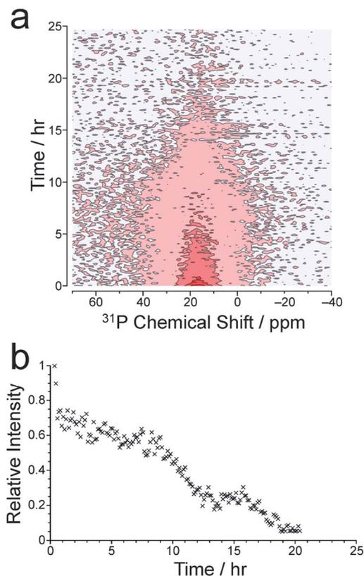
Fig. 2 (a) Intensity contour plot showing the time-dependence of the *in situ*  $^{31}\text{P}$  NMR spectrum (recorded without  $^1\text{H}$  decoupling) at 60 °C, representing the liquid-state  $^{31}\text{P}$  NMR signal. (b) Intensity vs. time plot for the liquid-state  $^{31}\text{P}$  NMR signal.
