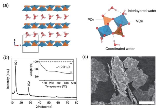
Fig. 1 (a) Crystal structure of VOPO<sub>4</sub>·*n*H<sub>2</sub>O. V (dark cyan), P (orange), O (red), and H (gray) atoms are shown. (b) Powder X-ray diffraction pattern and (c) scanning electron microscopy image of VOPO<sub>4</sub>·*n*H<sub>2</sub>O. The inset in (b) is the thermal gravimetric analysis profile of VOPO<sub>4</sub>·*n*H<sub>2</sub>O.
