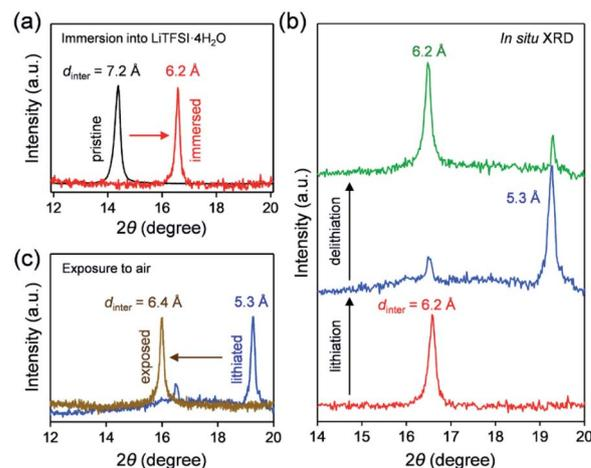
Fig. 4 Structural changes of  $\text{VOPO}_4 \cdot n\text{H}_2\text{O}$  in LiTFSI/4 $\text{H}_2\text{O}$ . The 001 diffraction peak (a) before and after immersion in LiTFSI/4 $\text{H}_2\text{O}$ , (b) after lithiation and delithiation in LiTFSI/4 $\text{H}_2\text{O}$ , and (c) before and after exposure of a lithiated sample to the ambient atmosphere.  $d_{\text{inter}}$  denotes the interlayer distance.
