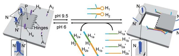
Fig. 4 Schematic pH-driven opening of the T-A·T triplex locked origami raft in the presence of the “helper” hairpins  $H_1$  and  $H_2$  to yield the nanocavity-containing tiles (at pH = 9.5) and their reversible closure at pH = 6.0 in the presence of the counter strands  $H'_{1a}/H'_{1b}$  and  $H'_{2a}/H'_{2b}$ .
