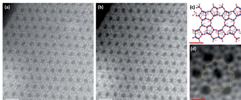
Fig. 3 Aberration-corrected HAADF-STEM image of Ag-ZSM-5 along the [010] axis. (a) Experimental image area (b) image is denoised using a nonlinear filtering algorithm (scale bar: 10 nm). (c) A structural model based on SXRD refinement, blue: Si or Al atoms as the TO<sub>4</sub> tetrahedra, and grey is silver ions. (d) Higher magnification of denoised HAADF-STEM image of Ag-ZSM-5; yellow dotted line label as a cyclic annular (scale bar: 8.15 Å).
