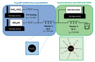
Fig. 1 Reaction setup for the continuous synthesis of  $Fe_3O_4NP$  and functionalization with NDA-PEG-COOH in a single set-up.  $t_R$  indicates the residence time in each reactor.
