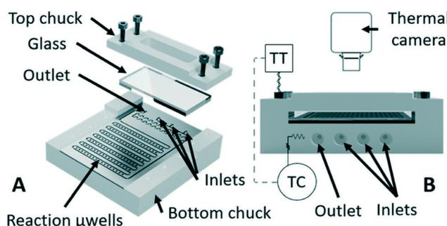
Fig. 10 Microreactor design adopted in Pd-catalyst assisted cross-linking reaction and relative mechanism study, main (A) and back (B) view of the reactor (adapted from ref. 44 copyright 2018 The Royal Society of Chemistry).
