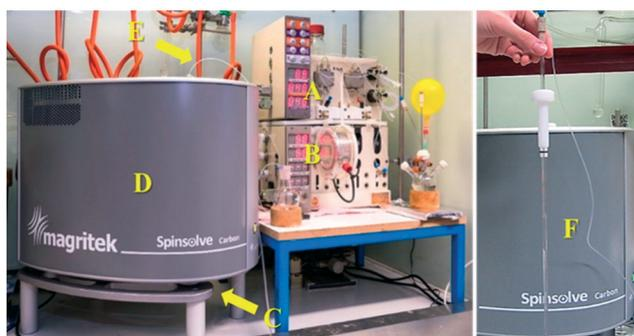
**Fig. 3** Robust platform for *in situ* reaction monitoring of a cyclopropanation reaction with Spinsolve benchtop NMR spectroscopy. (A) Vapourtec R2+ pump unit. (B) Vapourtec R4 reactor unit. (C) Flow stream input. (D) Benchtop NMR. (E) Flow stream output. (F) Glass NMR cell (adapted from ref. 33 copyright 2016 American Chemical Society).
