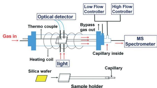
Fig. 11 Upper: The design of microreactor integrated with optical spectroscopic apparatus and sampling capillary (adapted from ref. 46 copyright 2015 American Chemical Society).
