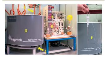
Fig. 3 Robust platform for in situ reaction monitoring cyclopropanation reaction with Spinsolve benchtop spectroscopy. (A) Vapourtec R2+ pump unit. (B) Vapourtec R4 reactor unit. (C) Flow stream input. (D) Benchtop NMR. (E) Flow stream output. (F) Glass NMR cell (adapted from ref. 33 copyright 2016 American Chemical Society).
