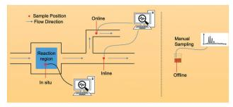
Fig. 1 Schematic illustration of in situ, inline, online and offline measurements
