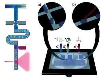
Fig. 9 Left: Schematic diagram of in situ Raman detection. Right: multichannel microfluidic chip, the flow-focussing (a) and dispensing structure (b) within microchannel. (c) reactant 1 inlet. (d) silver suspension inlet, (e) reactant 2 inlet (adapted from ref. 40 copyright 2015 The Royal Society of Chemistry).
