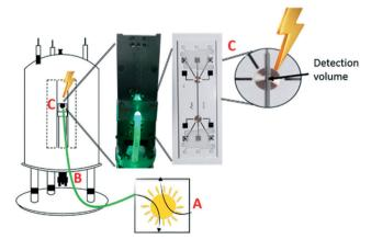
Fig. 4 Graphic representation of the assembly of nanolitre-in situ-NMR microfluidic chips. (A) UV-vis light source. (B) Non-contactsample optical fibre. (C) Sampling zone (adapted from ref. 34 copyright 2018 American Chemical Society).
