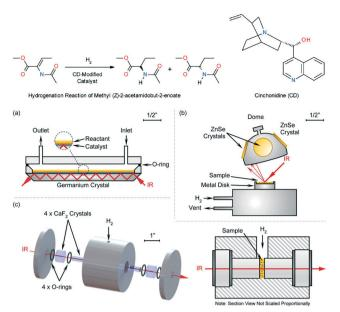
**Fig. 6** Upper: The hydrogenation of methyl (*Z*)-2-acetamidobut-2-enoate with a CD-doped Pd catalyst. Below: Detailed views of the *in situ* IR-microfluidics setup, (a) ATR infrared cell assembled by Ge crystal, (b) DRIFTS cell, (c) transmission FTIR structure (adapted from ref. 38 copyright 2016 American Chemical Society).
