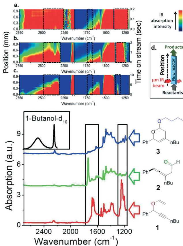
Fig. 5 Upper: Spatially resolved IR spectroscopic imaging along the flow reactor with various flow rates, 10 (a), 1 (b), 0.2 (c) mL h<sup>-1</sup>, respectively. (d) Scheme of microreactor for *in situ* IR and X-ray microspectroscopy measurements. Below: FTIR spectra of reactant, vinyl ether (red), allenic aldehyde (green), and acetal (blue) (adapted from ref. 37 copyright 2014 American Chemical Society).
