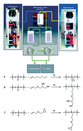
Fig. 7 Upper: Setup of *in situ* IR detection in flow reactors. Below: hydrosilylation of different olefins: (A) 1-octene, (B) 3-allyloxy-1,2-propanediol and (C) allyl glycidyl ether (adapted from ref. 39 copyright 2018 The Royal Society of Chemistry).
