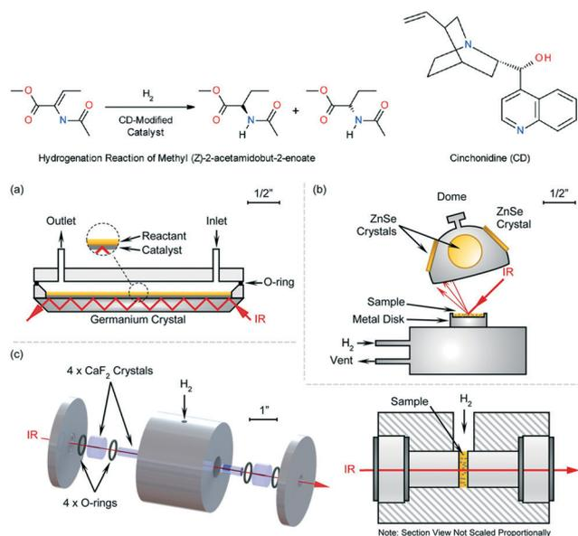
**Fig. 6** Upper: The hydrogenation of methyl (Z)-2-acetamidobut-2-enoate with a CD-doped Pd catalyst. Below: Detailed views of the *in situ* IR-microfluidics setup, (a) ATR infrared cell assembled by Ge crystal, (b) DRIFTS cell, (c) transmission FTIR structure (adapted from ref. 38 copyright 2016 American Chemical Society).
