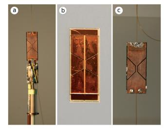
Fig. 2 Schematic view of three modified stripline chips for microfluidic flow NMR spectroscopy including 1D, 2D, and heteronuclear signals. (a) 100  $\mu m$  D263T borosilicate-made 165 nL volume chip with optimal resolution and sensitivity (b) 500  $\mu m$  fused silica-made 145 nL volume chip, preferable for small volume samples (c) borosilicate-made with a maximum volume of 215 nl. chip, similar design as (a) (adapted from ref. 26 copyright 2017 American Chemical Society).
