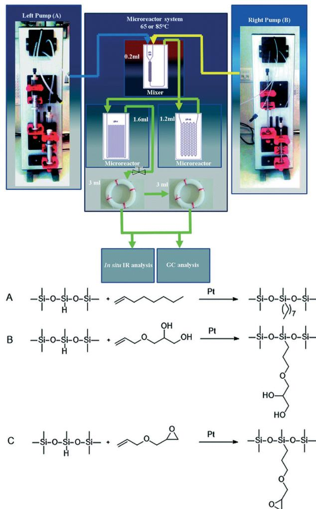
**Fig. 7** Upper: Setup of *in situ* IR detection in flow reactors. Below: hydrosilylation of different olefins: (A) 1-octene, (B) 3-allyloxy-1,2-propanediol and (C) allyl glycidyl ether (adapted from ref. 39 copyright 2018 The Royal Society of Chemistry).
