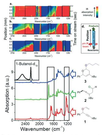
Fig. 5 Upper: Spatially resolved IR spectroscopic imaging along the flow reactor with various flow rates, 10 (a), 1 (b), 0.2 (c) mL  $h^{-1}$ , respectively. (d) Scheme of microreactor for in situ IR and X-ray microspectroscopy measurements. Below: FTIR spectra of reactant, vinyl ether (red), allenic aldehyde (green), and acetal (blue) (adapted from ref. 37 copyright 2014 American Chemical Society).
