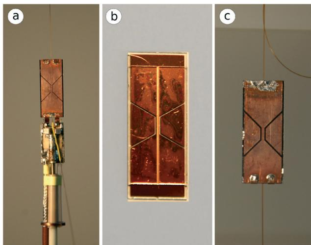
**Fig. 2** Schematic view of three modified stripline chips for microfluidic flow NMR spectroscopy including 1D, 2D, and heteronuclear signals. (a) 100  $\mu\text{m}$  D263T borosilicate-made 165 nL volume chip with optimal resolution and sensitivity (b) 500  $\mu\text{m}$  fused silica-made 145 nL volume chip, preferable for small volume samples (c) borosilicate-made with a maximum volume of 215 nL chip, similar design as (a) (adapted from ref. 26 copyright 2017 American Chemical Society).
