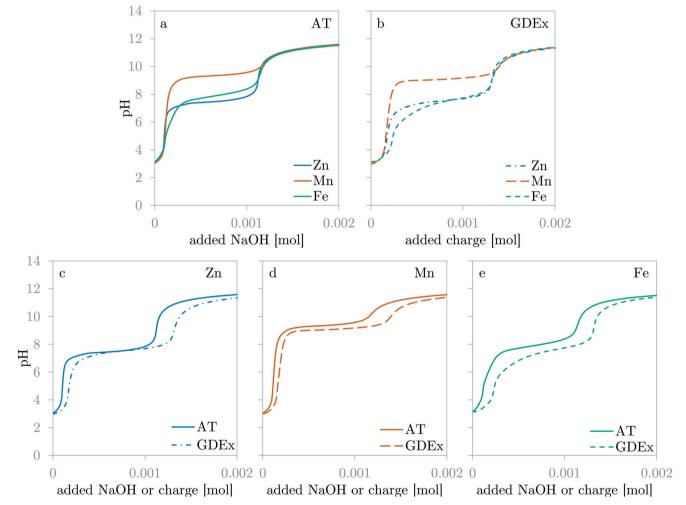
Fig. 5 Comparison of the dynamic pH curves for ZnCl<sub>2</sub>, MnCl<sub>2</sub> and FeCl<sub>2</sub> for AT (a) and GDEx (b). Comparison of the dynamic pH curves for AT and GDEx for ZnCl2 (c), MnCl2 (d) and FeCl2 (e).
