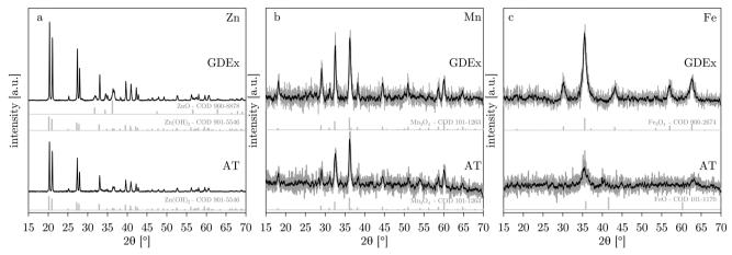
Fig. 7 XRD patterns for AT and GDEx for solutions with ZnCl<sub>2</sub> (a), MnCl<sub>2</sub> (b) or FeCl<sub>2</sub> (c). XRD reference patterns (from the crystallography open database - COD<sup>42-47</sup>) are shown below the AT and GDEx patterns for the detected phases.
