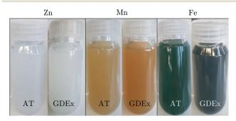
Fig. 3 Photographs of dispersed precipitates collected as-is from the AT and GDEx processes of ZnCl2, MnCl2, or FeCl2.
