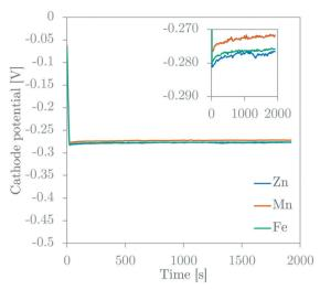
Fig. 6 Potentiograms of galvanostatic GDEx experiments for solutions with ZnCl2, MnCl2 or FeCl2. Insert gives a comparison in a smaller potential range.
