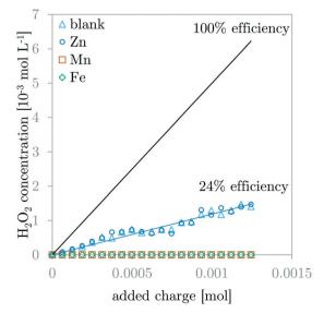
Fig. 4 Comparison of H<sub>2</sub>O<sub>2</sub> concentration measurements during GDEx experiments of a blank solution and solutions with ZnCl<sub>2</sub>, MnCl<sub>2</sub>, or  $FeCl_2$ . The  $H_2O_2$  production efficiency (24%) for the case of the blank solution and the ZnCl<sub>2</sub> solution are the same (blue interpolation line). The 100% efficiency line is indicated for comparison.
