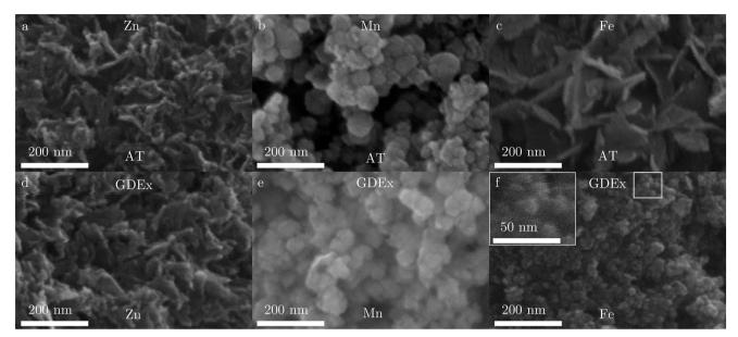
Fig. 8 SEM images of the precipitates synthesized with AT (a-c) and GDEx (d-f) for the cases of ZnCl<sub>2</sub> (a and d), MnCl<sub>2</sub> (b and e), and FeCl<sub>2</sub> (c and f).
