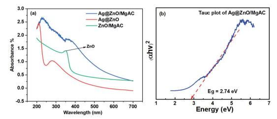
Fig. 3 (a) UV-Vis absorption spectrum of ZnO/MgAC, Ag@ZnO, and Ag@ZnO/MgAC nanocomposites; (b) energy band gap estimation through the results of the Tauc plot of Ag@ZnO/MgAC.
