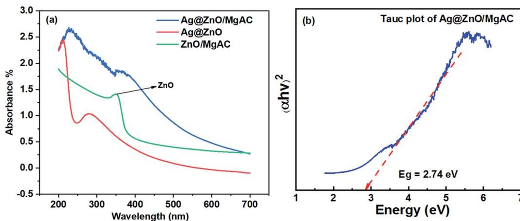
Fig. 3 (a) UV-Vis absorption spectrum of ZnO/MgAC,  $\text{Ag@ZnO}$ , and  $\text{Ag@ZnO/MgAC}$  nanocomposites; (b) energy band gap estimation through the results of the Tauc plot of  $\text{Ag@ZnO/MgAC}$ .
