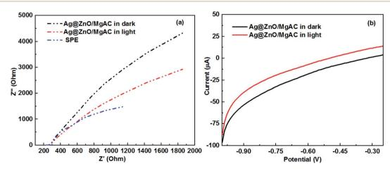
Fig. 6 (a) Nyquist plots of SPE and Ag@ZnO/MgAC/SPE electrodes and (b) linear scan voltammograms obtained for Ag@ZnO/MgAC/SPE electrodes under dark and visible light irradiations.
