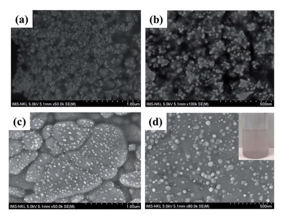
Fig. 4 SEM images of the synthesized Ag@ZnO samples (a and b); and Ag@ZnO/MgAC sample (c and d). The inset of (d) shows Ag@ZnO/MgAC sample image after storing for 3 days.
