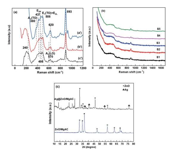
Fig. 2 (a and b) Raman spectra of ZnO/MgAC (a'), Ag@ZnO (b'), and the different Ag@ZnO/MgAC (c') samples synthesized at various conditions; (c) XRD results of ZnO/MgAC and Ag@ZnO/MgAC samples.
