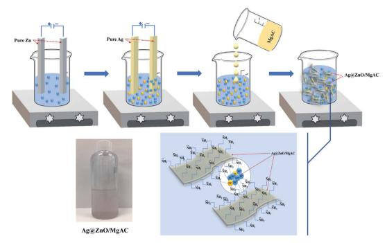
Fig. 1 Schematic illustrations for the synthesis of Ag@ZnO/MgAC nanocomposite design using the electrochemical method.
