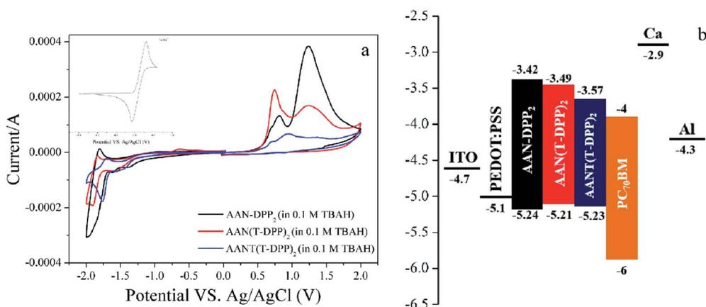
Fig. 3 (a) CV curves of SMs at a scan rate of 50 mV s<sup>-1</sup> and (b) schematic energy diagram of the materials used in the SM-OSCs.
