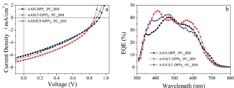
Fig. 6 (a)  $J$ - $V$  curves and (b) EQE spectra of the SMs/PC<sub>71</sub>BM cells at the optimized SMs/PC<sub>71</sub>BM devices under AM1.5 G illumination (100 mW cm<sup>-2</sup>).
