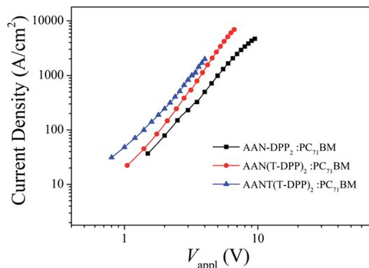
Fig. 5  $J$ - $V$  curve of the hole-only SMs: PC<sub>71</sub>BM-based devices under the optimized processing conditions.
