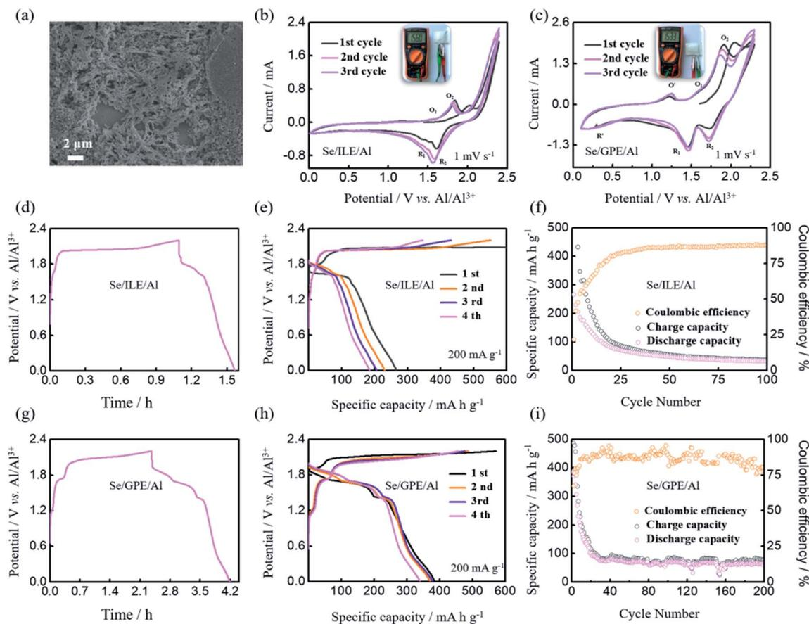
Fig. 2 (a) FESEM image of positive electrode before cycling. (b and c) The initial three CV curves at a scan rate of  $1 \text{ mV s}^{-1}$  of Al–Se batteries with ILE and GPE. (d and g) The charge/discharge profiles of Al–Se batteries with ILE and GPE. (e and h) The charge/discharge curves at  $200 \text{ mA g}^{-1}$  of Al–Se batteries with ILE and GPE. (f and i) The corresponding cycling performance and coulombic efficiency with ILE and GPE.
