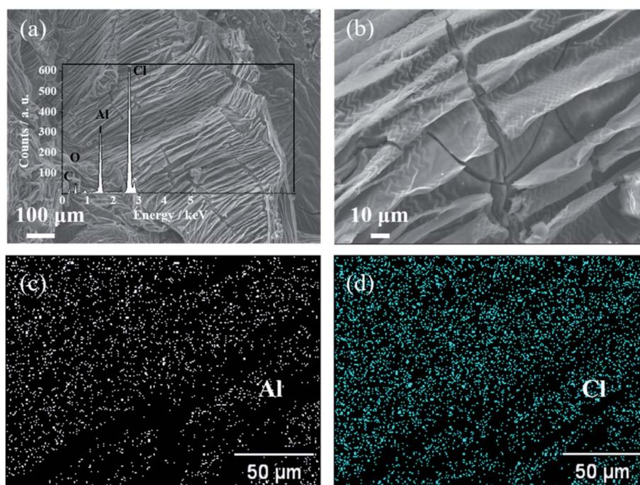
Fig. 5 (a and b) FESEM images of the 50<sup>th</sup> cycled GPE. Inset: the corresponding EDS spectrum of cycled GPE. (c and d) EDS mapping images of Al and Cl of the 50<sup>th</sup> cycled GPE.
