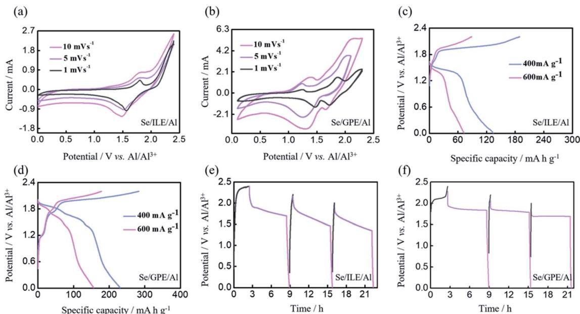
Fig. 3 (a and b) The CV curves at scan rates of 1, 5, 10  $\text{mV s}^{-1}$  of Al–Se batteries with ILE and GPE. (c and d) The charge/discharge curves at 400 and 600  $\text{mA g}^{-1}$  of Al–Se batteries with ILE and GPE. (e and f) The self-discharge behaviors of Al–Se batteries with ILE and GPE under different charge potentials.
