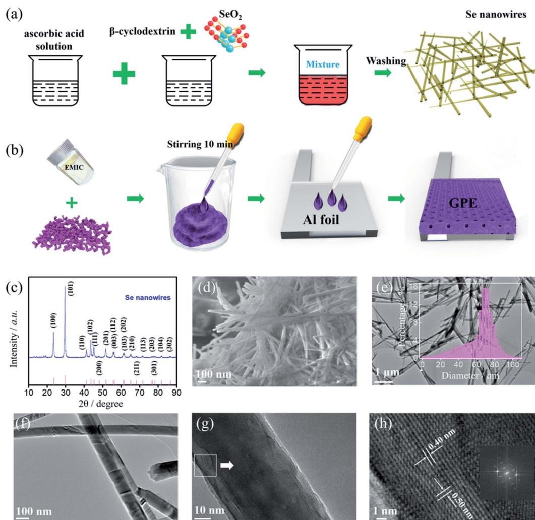
Fig. 1 (a) Schematic diagram of the preparation of selenium nanowires. (b) Schematic diagram of the preparation of the GPE. (c) XRD pattern of as-prepared selenium nanowires. (d) FESEM images of selenium nanowires. (e and f) TEM images of selenium nanowires. Inset: the histogram of Se nanowires diameter. (g and h) HRTEM images of selenium nanowires.
