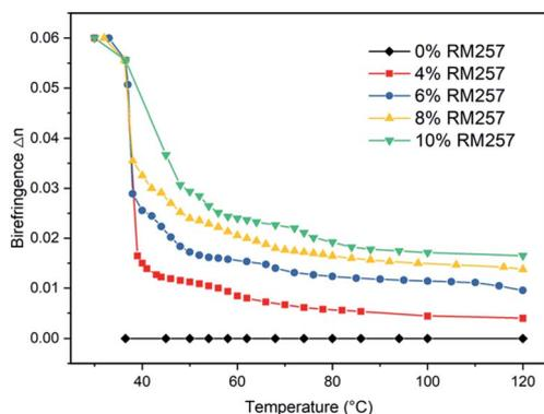
Fig. 7 Birefringence ( $\Delta n$ ) of the PNLC with different concentrations of RM257 at different temperatures from 36 °C to 120 °C. The estimated  $\Delta n$  values were obtained from the colorimetric responses shown in Fig. 6 according to the Michel-Levy chart.
